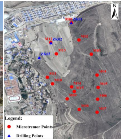
Fig. 1 – The Full View of Subao Landslide (Lens pointing, 165° ) Fig. 2 – Drilling and Microtremor Points
