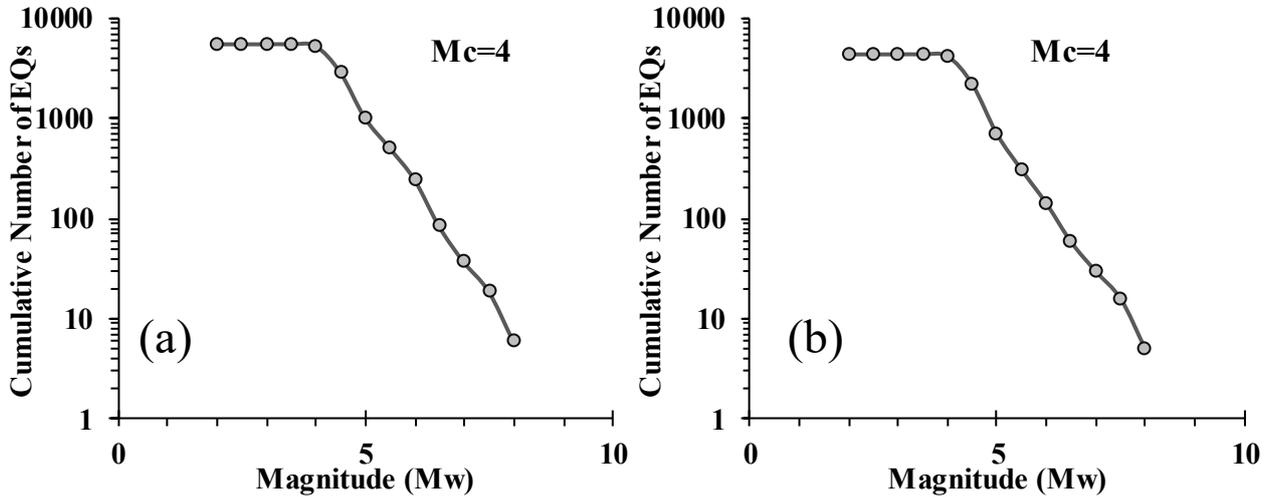
Fig. 2 – Cumulative frequency distribution plots and  $M_c$  values for (a) the catalogue before declustering and (b) for the catalogue after declustering
