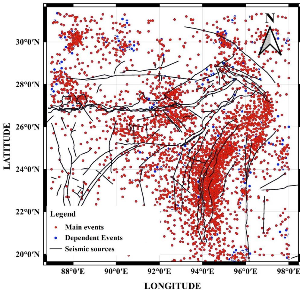
Fig. 6 – Seismic sources in NE India region along with EQ data from both catalogue before declustering and catalogue after declustering
