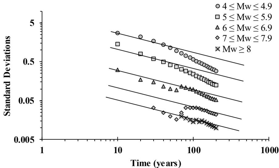
Fig. 4 – Standard deviation versus time interval plots for different magnitude classes catalogue after declustering
