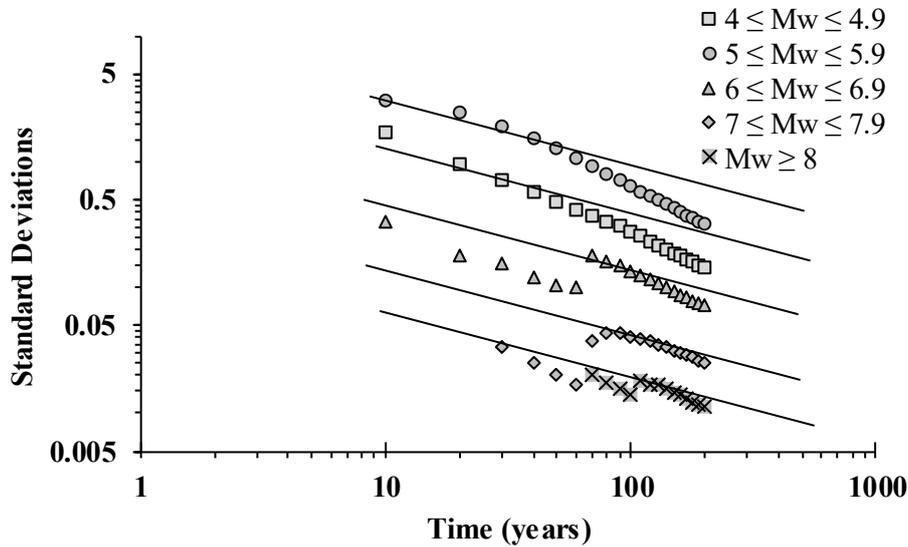
Fig. 3 – Standard deviation versus time interval plots for different magnitude classes for the EQ catalogue before declustering
