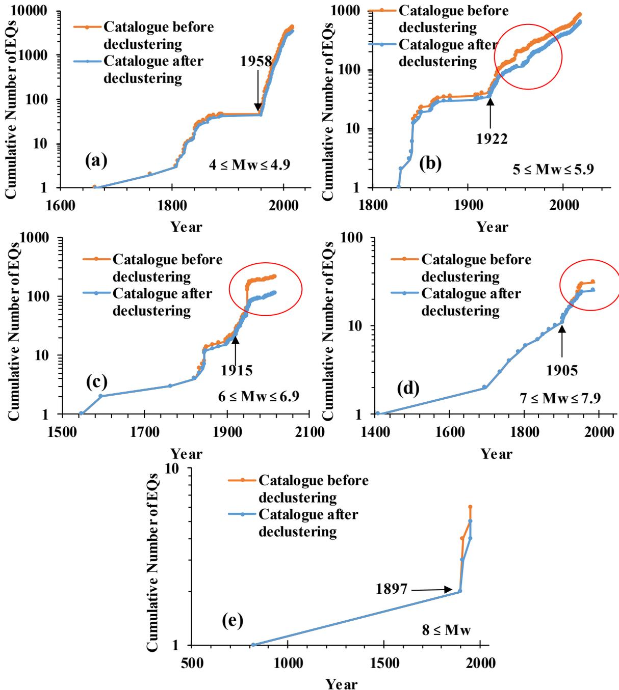
Fig. 5 – CUVI method for determining catalogue completeness (arrow showing the point after which the data are complete with respect to time)
