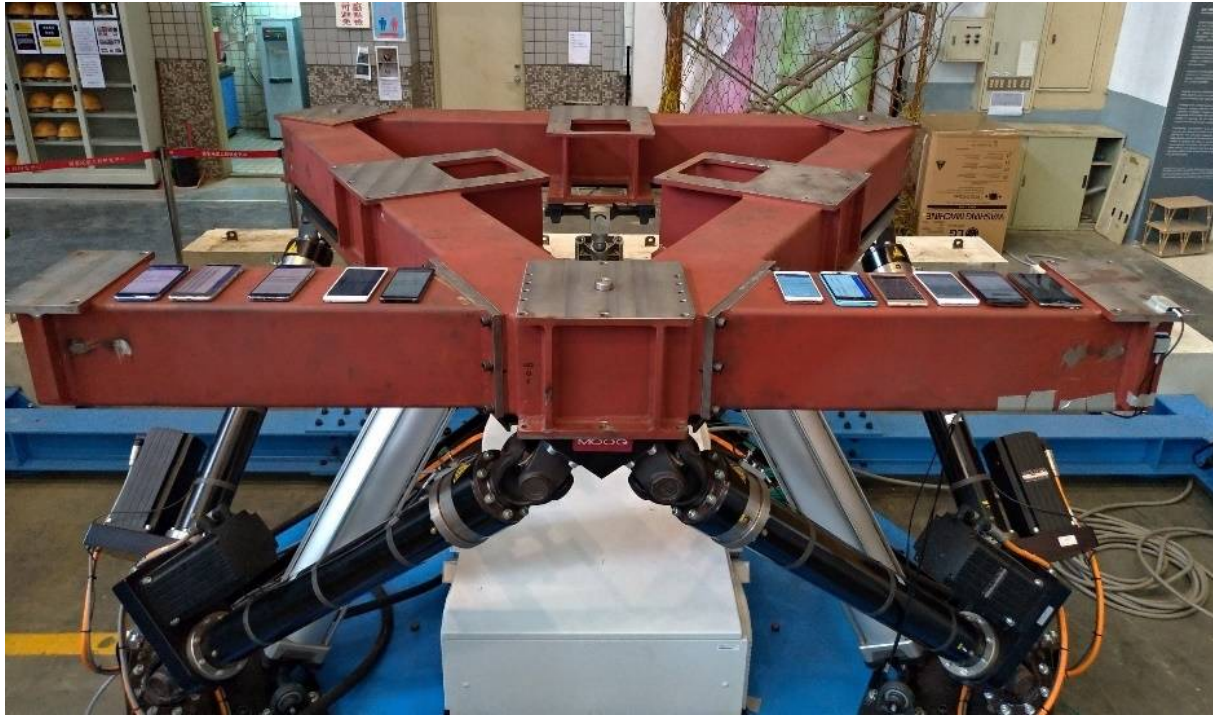
Fig. 3 – Test setup of the shaking table tests.
