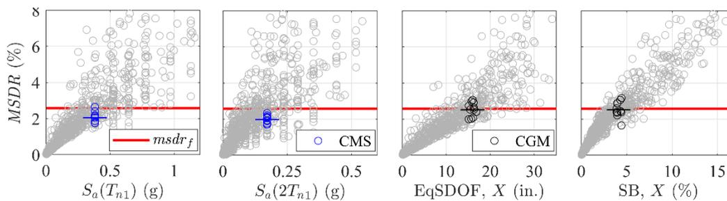
Fig. 7 - Relation between *MSDR*, and different response predictors for the eight-story special moment frame
