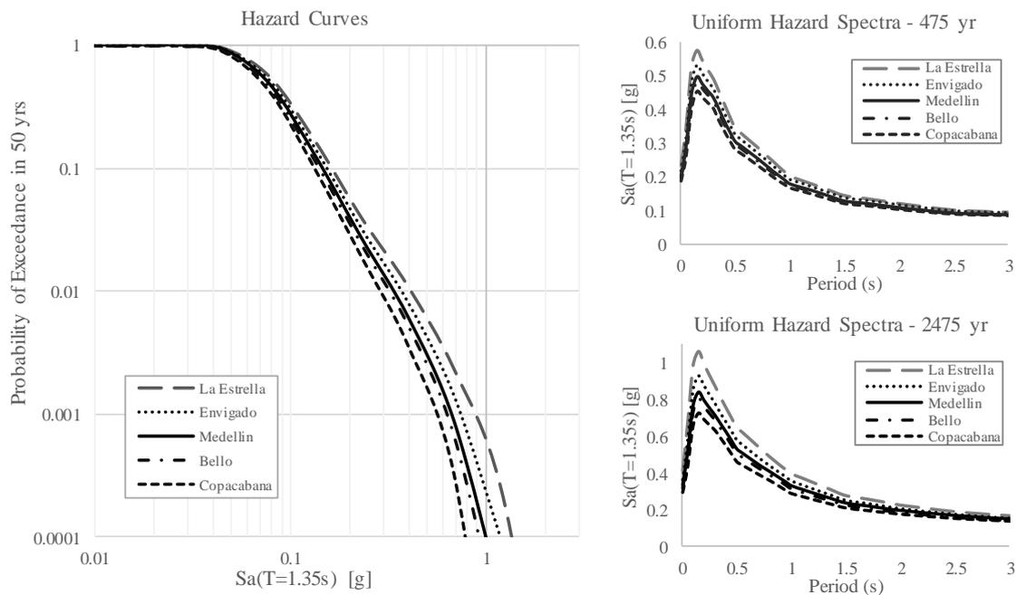
Fig. 4 - Hazard curves for the five cities and uniform hazard spectra for return periods of 475 and 2475 years.
