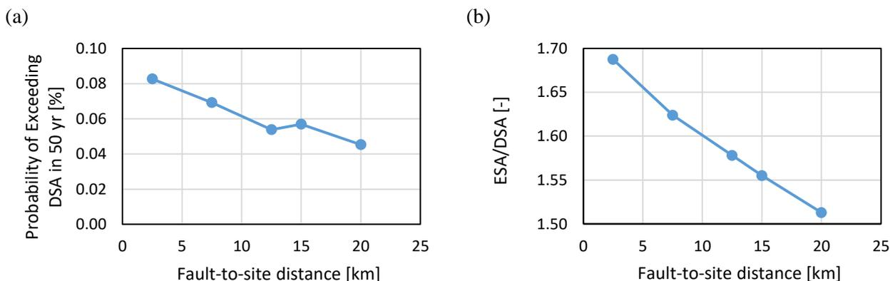
Fig. 9 – (a) Probability of exceeding the design spectral acceleration in 50 yr and. (b) Expected over design spectral acceleration as a function of the distance to the fault.
