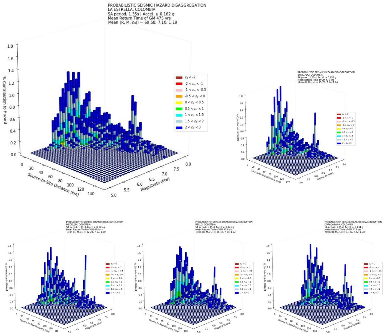
Fig. 5 - Seismic hazard disaggregation for the five cities, La Estrella, Envigado, Medellin, Bello, and Copacabana, at  $S_a(T=1.35s)$  for 475 year return period.
