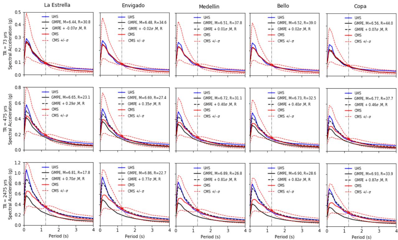
Fig. 6 - Conditional Mean Spectrum for the cities of La Estrella, Envigado, Medellin, Bello y Copacabana, return periods of 73, 475 and 2475 years, Romeral fault source at  $T^* = 1.35s$ .
