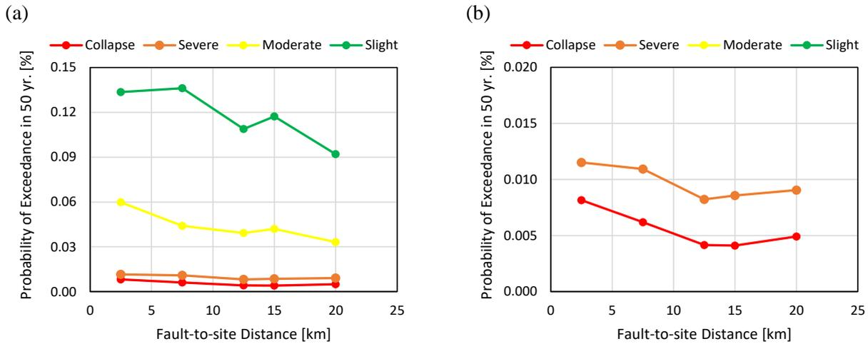
Fig. 10 – Probability of exceeding the slight, moderate, severe and collapse limit states in 50 years.
