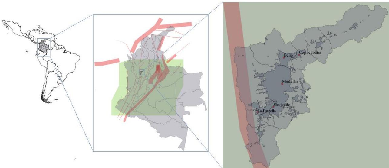
Fig. 1 - Seismic sources of the hazard model used (red: active shallow-crust; green: subduction [3]) and location of cities under study
