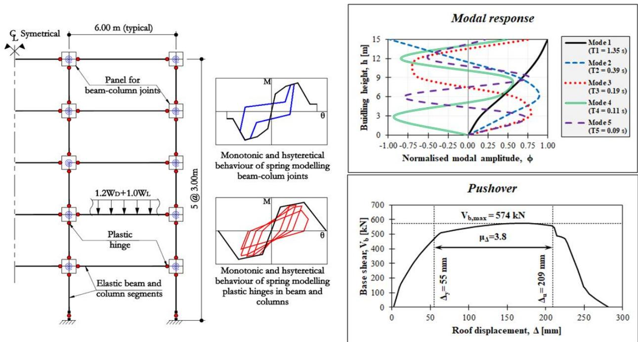
Fig. 3 - Analytical model scheme (left) and main features of the structural response of the case study structure (right).
