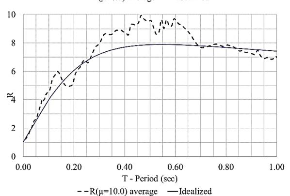
Fig. 7: Comparison of strength reduction factors between the average data and the idealized proposal for different ductility demand values.
