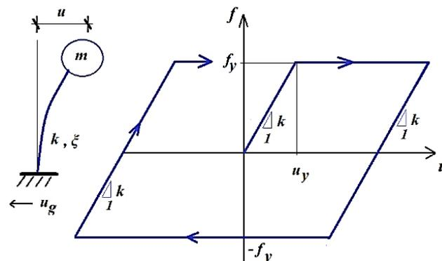
Fig. 2: SDOF system for analysis and elastic-plastic behavior considered.
