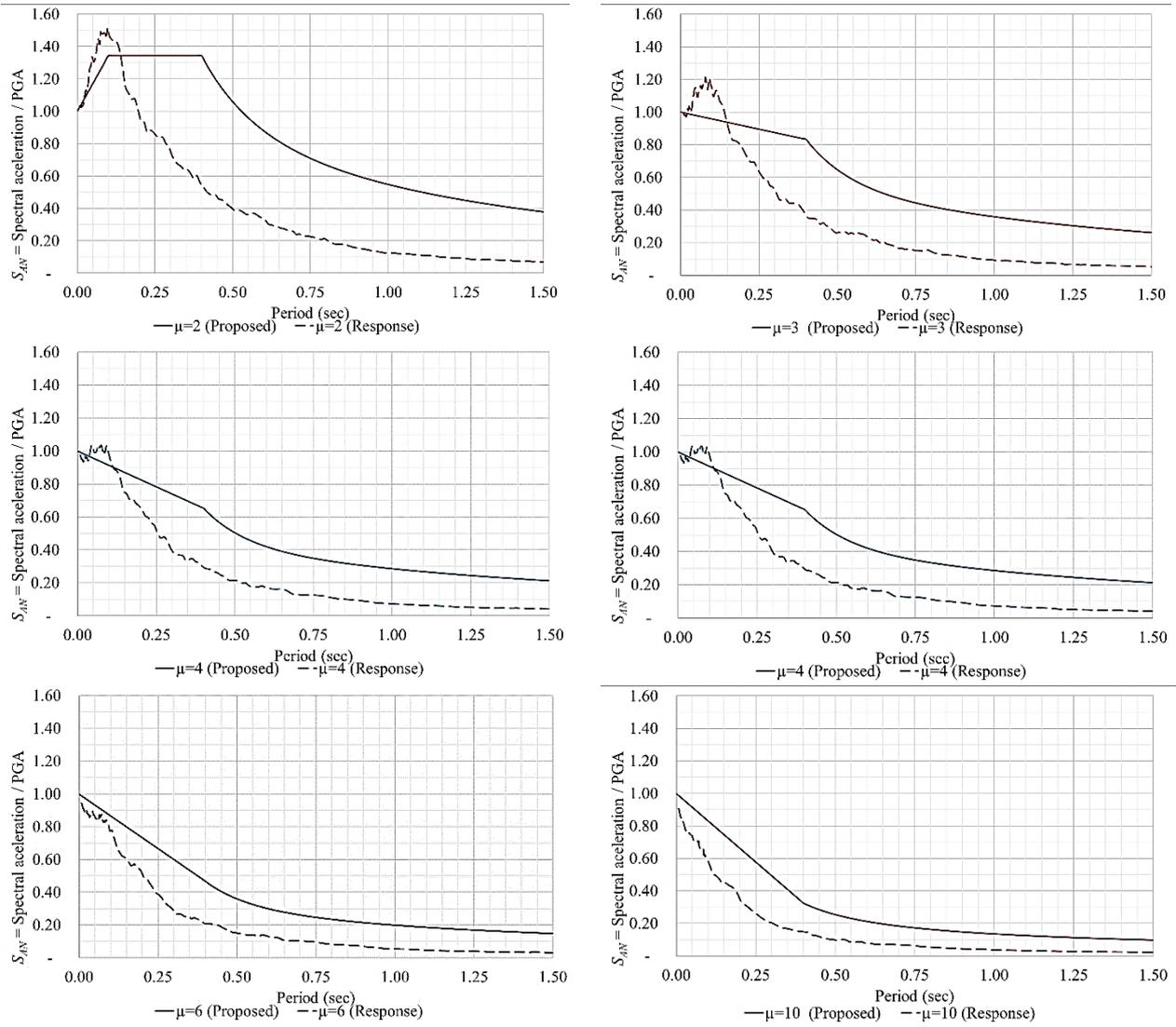
Fig. 8: Comparison of proposal design spectrum and response from data for different ductility values.
