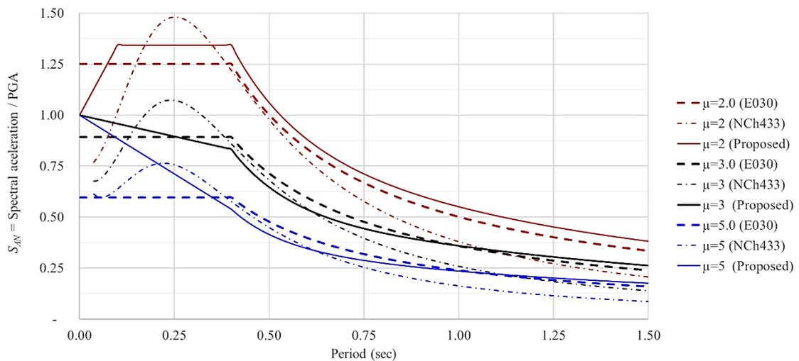
Fig. 9: Comparison of inelastic design spectrum of Peruvian Code (E030), Chilean code (NCh433) and spectrum proposed for ductility values of 2.0, 3.0 and 5.0.
