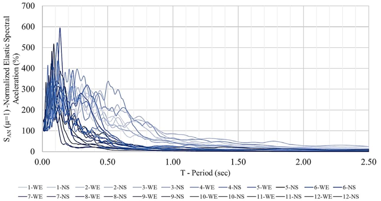
Fig. 3: Normalized Elastic Spectral Acceleration Responses for the 24 signals processed  $S_{AN}(\mu=1)$ .
