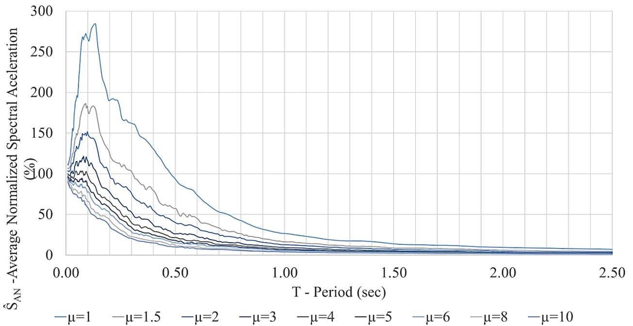
Fig. 4: Average Normalized Spectral Acceleration associated with the predetermined ductility factor values  $\hat{S}_{AN}(\mu = \mu_i)$ .
