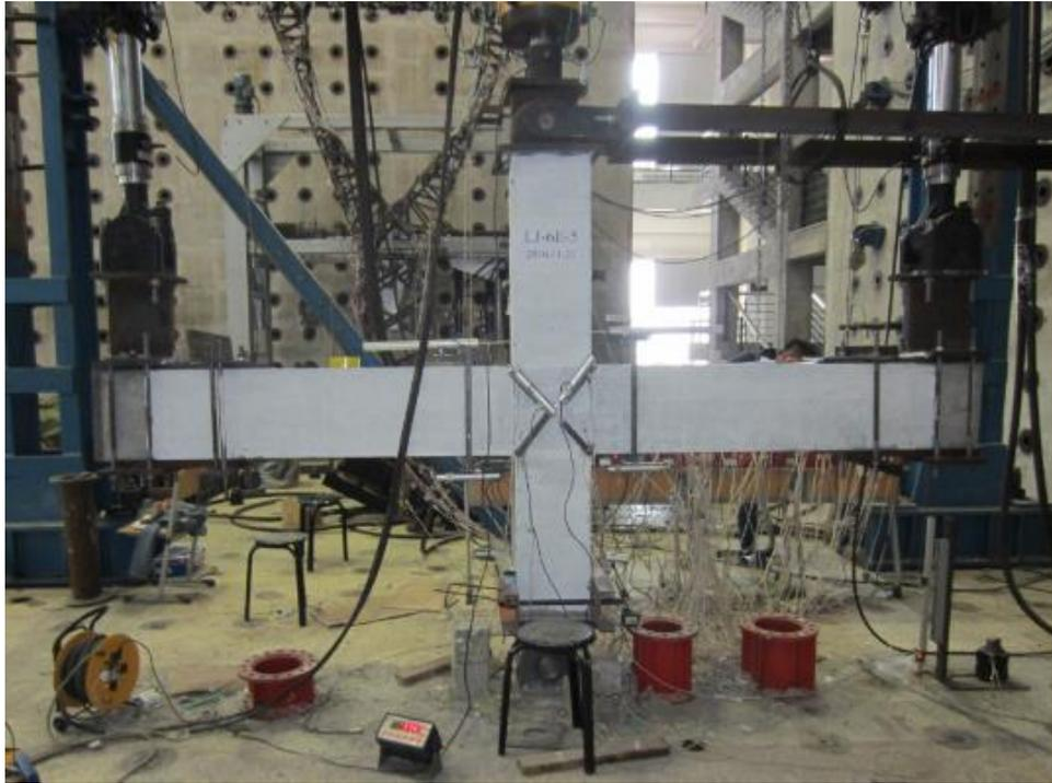
Fig. 2 – Loading apparatus
