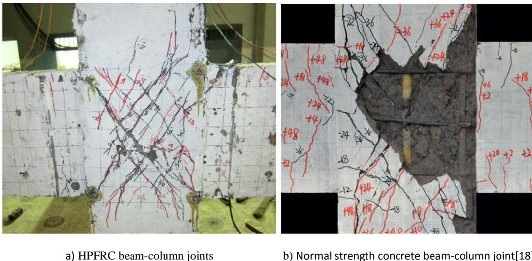
Fig. 3 – Failure patterns of beam-column joint.
