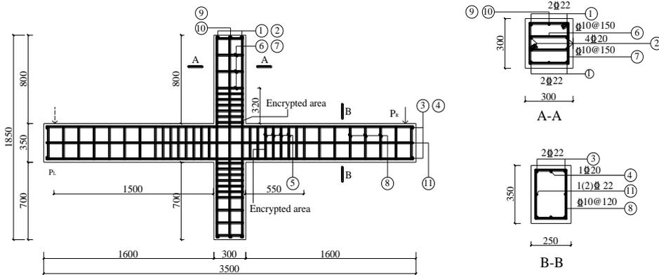
Fig. 1 – Details of geometry and reinforcement of the specimens
