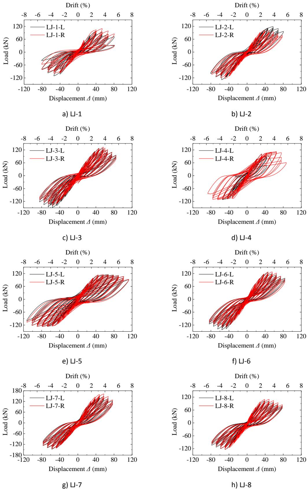
Fig. 4 – Hysteretic curve of specimens
