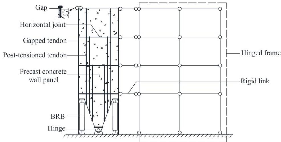
Fig. 8 – HWBB with gapped tendons-hinged frame structure
