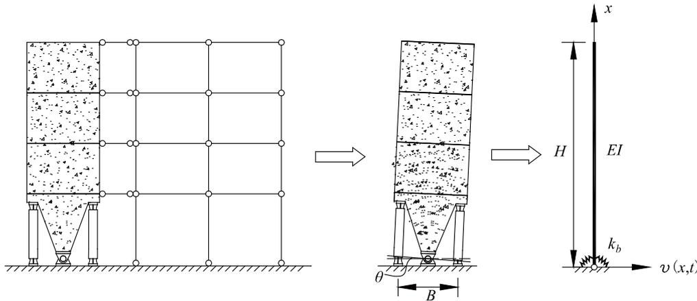
Fig. 5 – Simplified model of the HWBB-hinged frame structure
