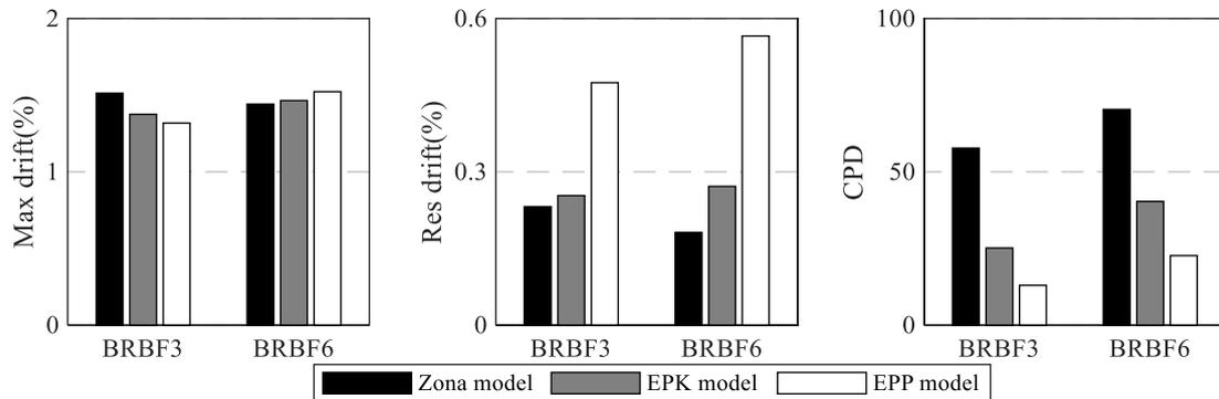
Fig. 6 – Comparison of seismic demands on BRBF subject to DBE earthquakes
