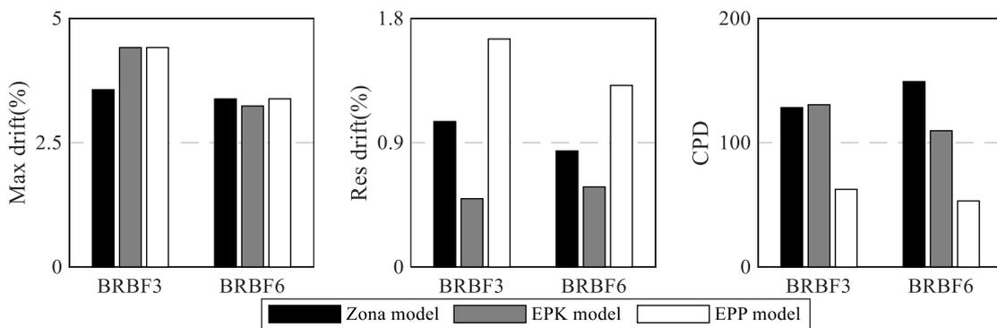
Fig. 7 – Comparison of seismic demands on BRBF subject to MCE earthquakes
