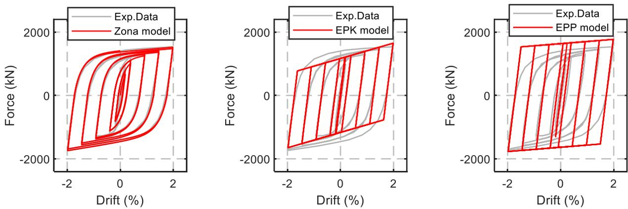
Fig. 4 – Simulation results of different hysteretic models
