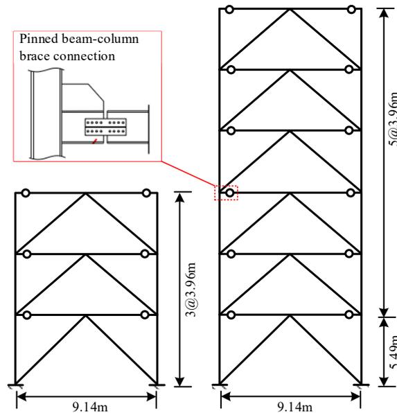
Fig. 3 – Elevation view of bare BRBF
