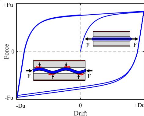
Fig. 1 – Characteristics of the BRB hysteretic behaviour
