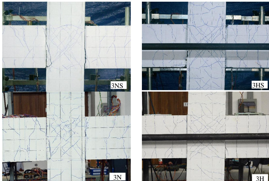
Fig.10 - Damage condition of specimens at 2% lateral drift.
