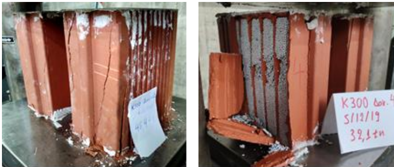
Figure 12: Modes of failure observed after compression test for the bare brick (left) and the filled with EPS brick (right)
