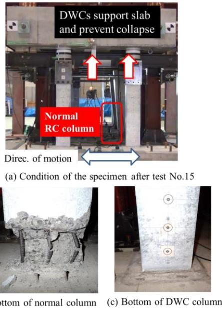
Fig. 4 – General view of the specimen after tests
