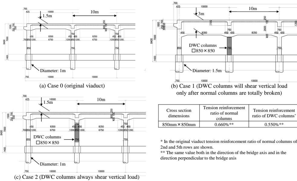
Fig. 9 – Structural specifications of the viaducts based on the design
