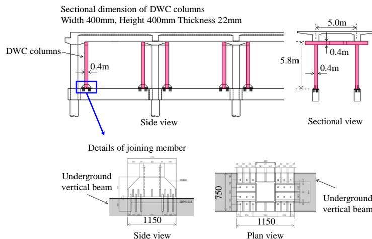
Fig. 12 – Structural specifications of the DWC columns installed in existing viaducts
