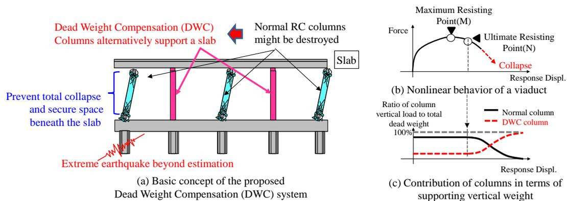
Fig. 1 – Schematic view of dead weight compensation structure [1, 3 (partially corrected)]
