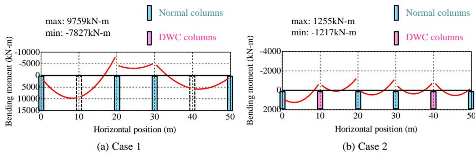
Fig. 10 – Bending moment diagrams of the vertical beams in the ordinary condition
