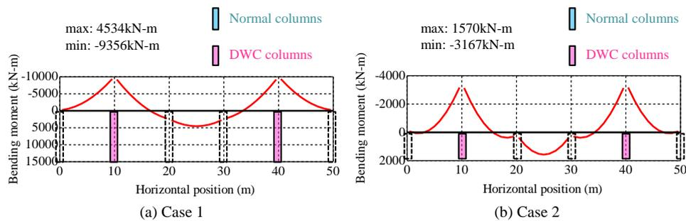
Fig. 11 – Bending moment diagrams of the vertical beams after normal columns have broken totally
