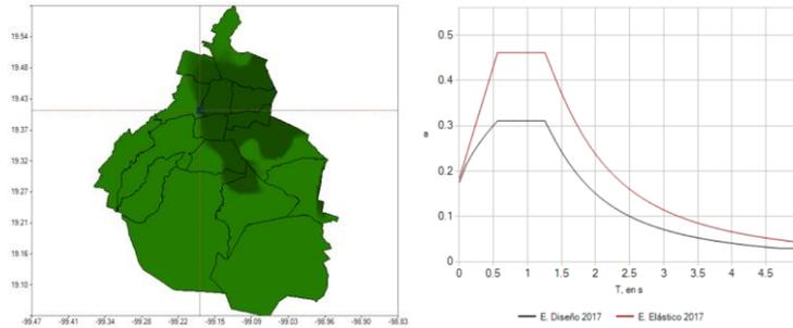
Fig. 4 – Seismic zoning and design spectrum of building 1
