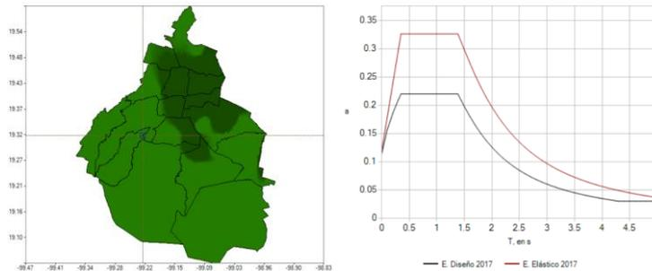
Fig. 2 – Seismic zoning and design spectrum of building 1
