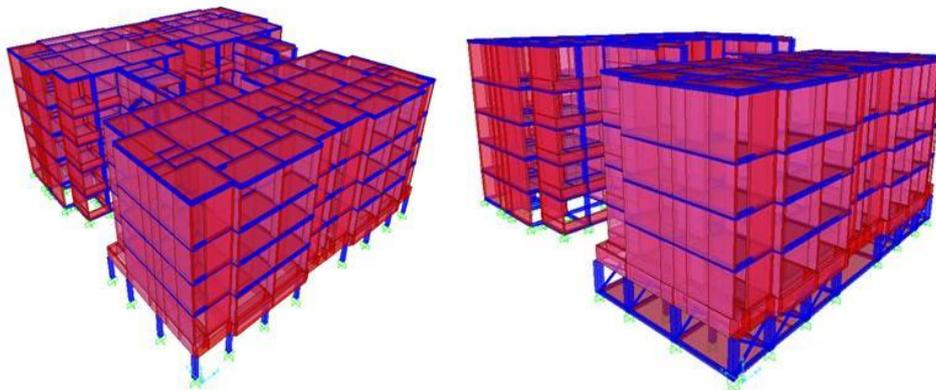
Fig. 5 – Original and reinforced structural models of building 3 with “weak ground floor”
