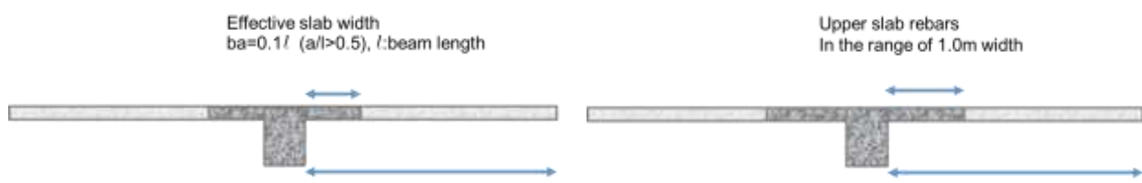
(a) Effective slab width for the first phase design (b) Effective slab width for the second phase design Fig. 1 – Effective slab width for beams in the Japanese seismic design code of practice
