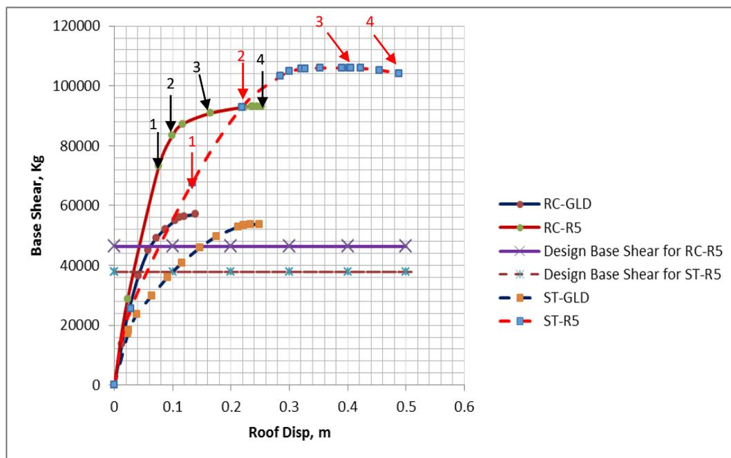
Fig. 7 - Comparisons of base shear capacity and roof displacement between masonry infilled reinforced concrete buildings (RC) and steel buildings (ST) for intermediate ductile frames (IDF) with R=5 and gravity load designed (GLD) frames
