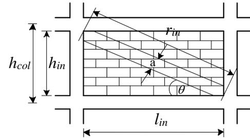
Fig. 4 - Equivalent diagonal compression strut model
