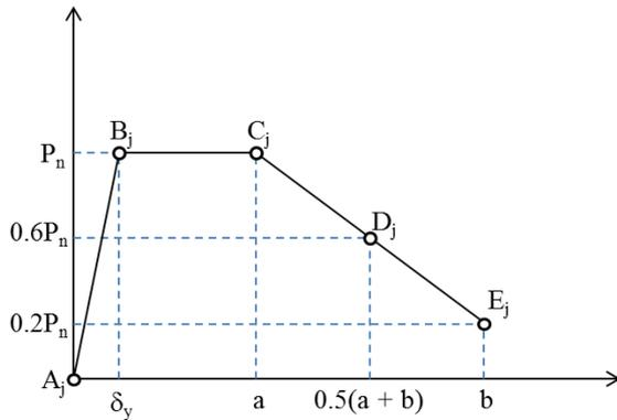
Fig.3 - Behavior of the PH of a beam-column joints.
