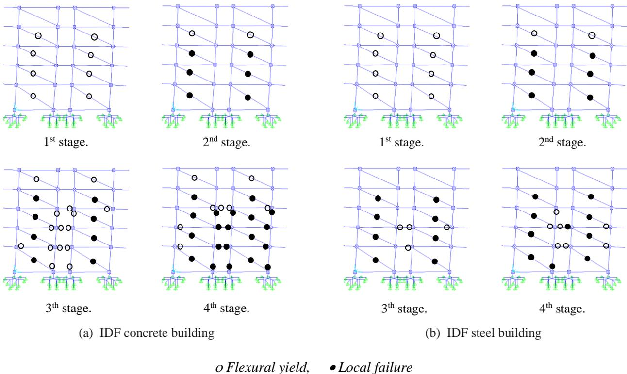
Fig. 8 - Hinge mechanism patterns in IDF concrete and steel buildings (see with Fig. 7).
