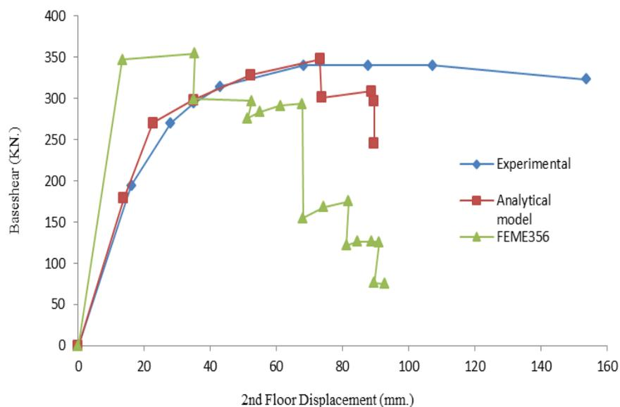
Fig. 6 - Comparisons between pushover curves and experiments for Vecchio and Emara Frame [14].
