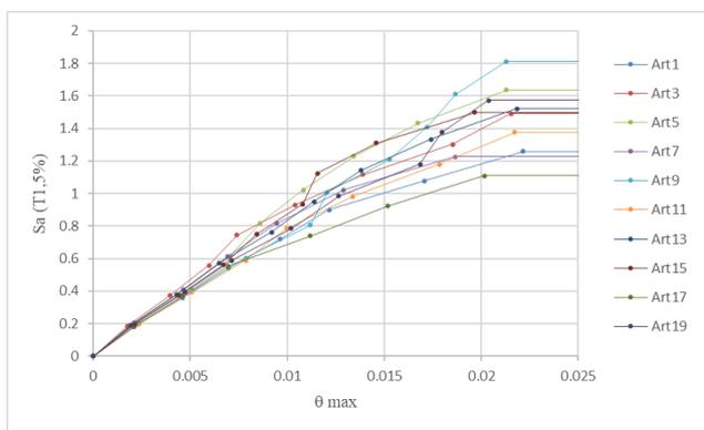
b.) Intermediate ductile frames, R = 5
