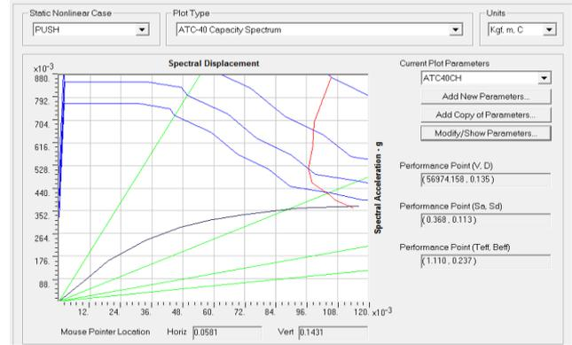
Fig.13: Performance point of GLD concrete building at collapse stage by capacity spectrum method
