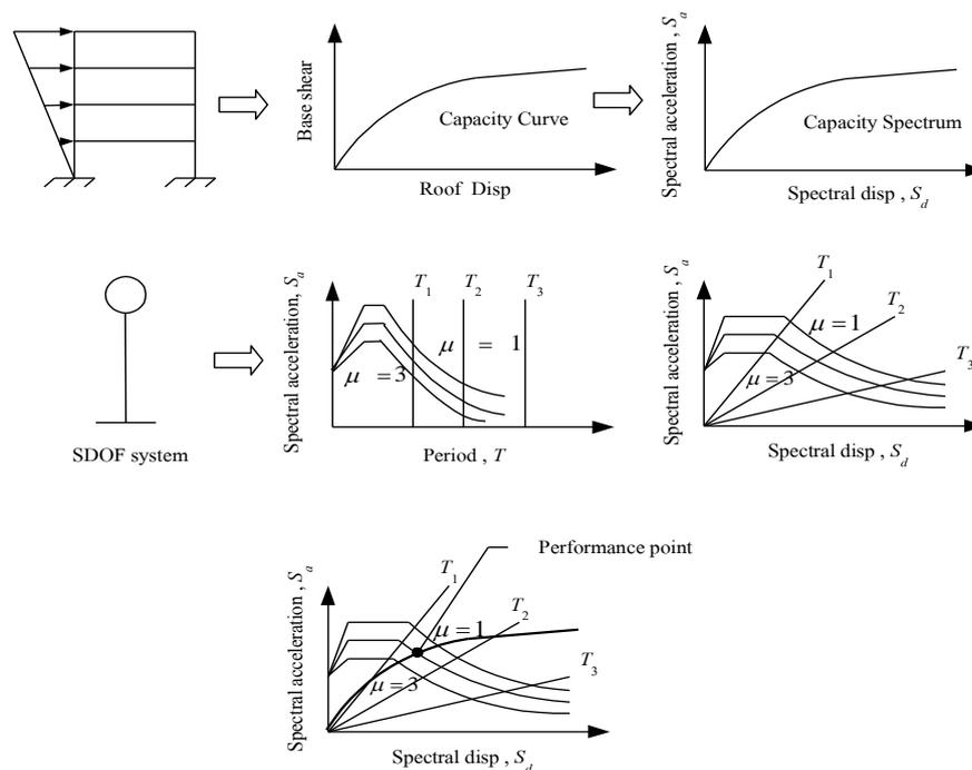
Fig. 11 - The procedure of CSM to estimate of the response of the structure
