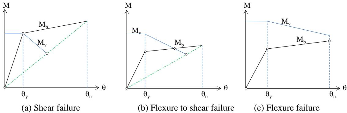
Fig. 2 - Failure modes of a column or beam and their plastic hinge characteristics.
