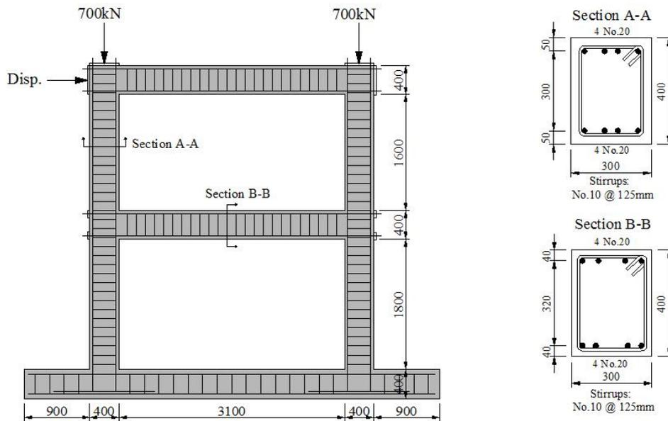
Fig. 5 - Details of Vecchio and Emara Frame for experiments [14].
