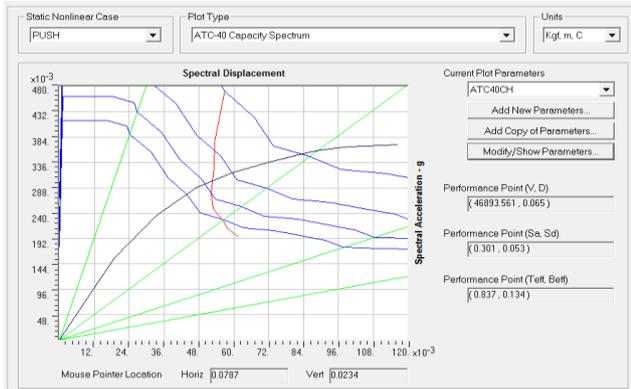
Fig.12: Performance point of GLD concrete building at yield stage by capacity spectrum method
