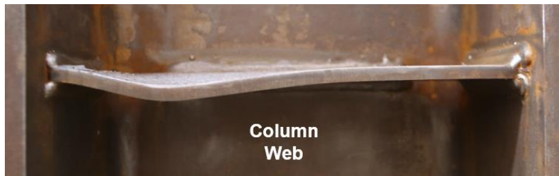
Fig. 8 – Continuity Plate Instability (Specimen C5)
