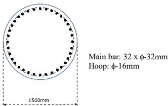
Fig. 15 – Revised cross-section (Case 1)
