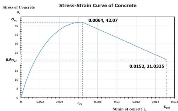
Fig.5 – Stress-strain relation of concrete
