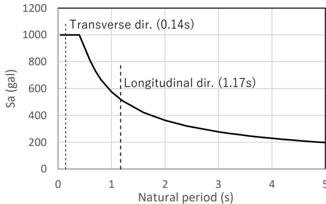
Fig.4 – Design acceleration response spectrum
