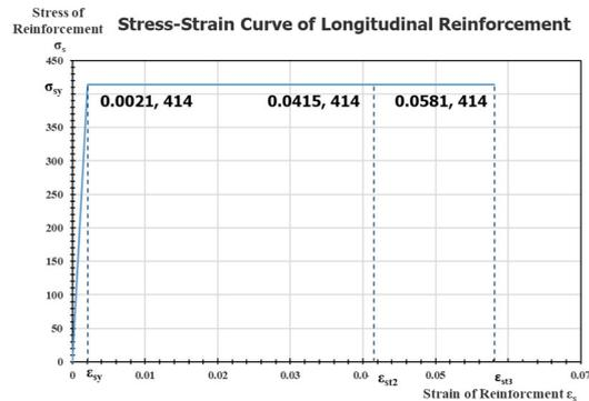
Fig.6 – Stress-strain relation of steel bar
