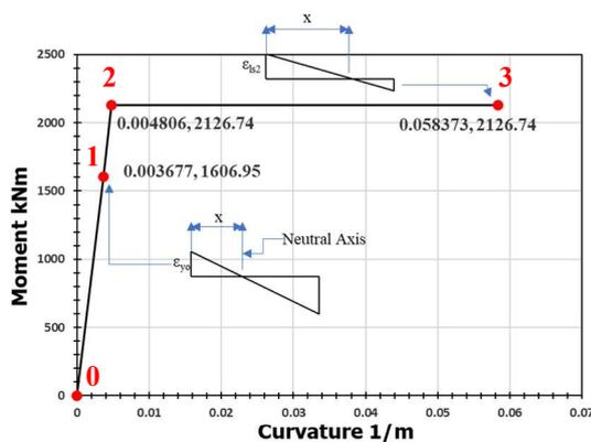
Fig.7 – M– $\phi$  relation of pier section
