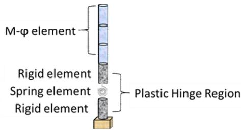
Fig.10 – Simple numerical model
