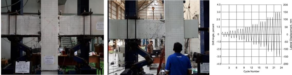
Fig. 19 – Beam column joint test
