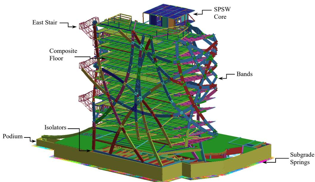
Fig. 11 3D Isometric view of the LS-DYNA analysis model of the (W)rapper Tower [9]
