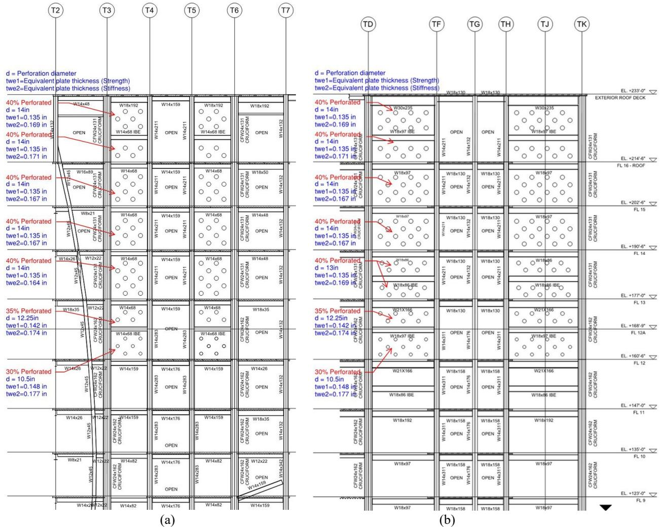
Fig. 12 – Selected perforation pattern for SPSWs along Tower height at (a) EW and (b) NS directions.
