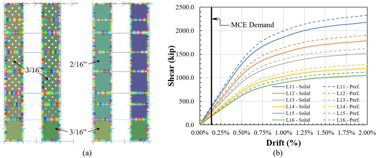
Fig. 13 – FEA model (a) in EW direction and (b) comparisons of pushover curves
