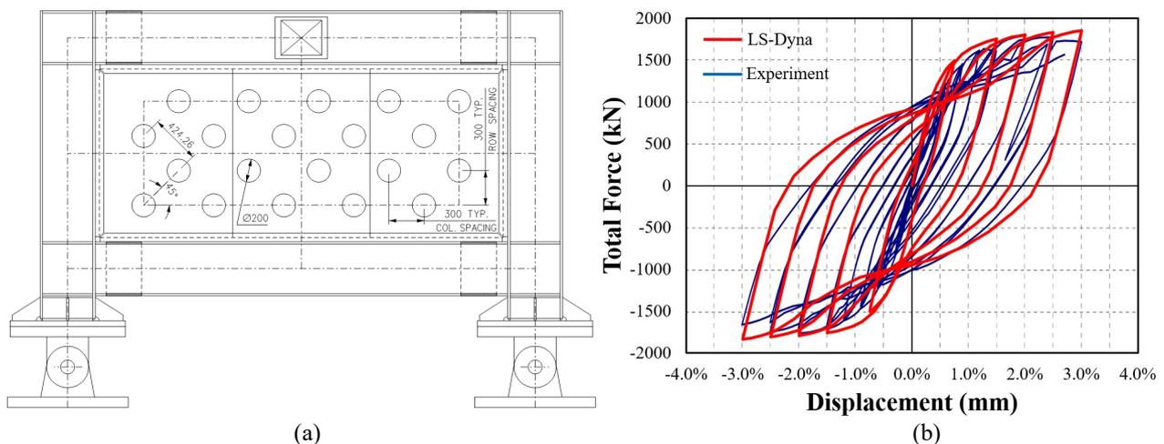
Fig. 5 – Perforated SPSW test specimen (a) and comparison of hysteresis response curves (b)
