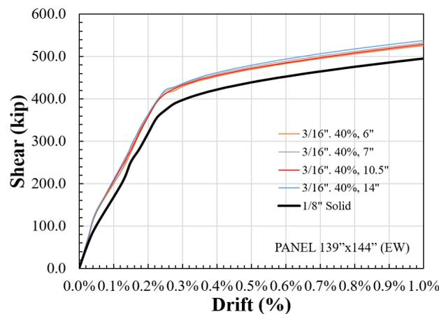
Fig. 9 – Pushover of a single panel with 40% perforation ratio with holes varying from 6” to 14” in diameter
