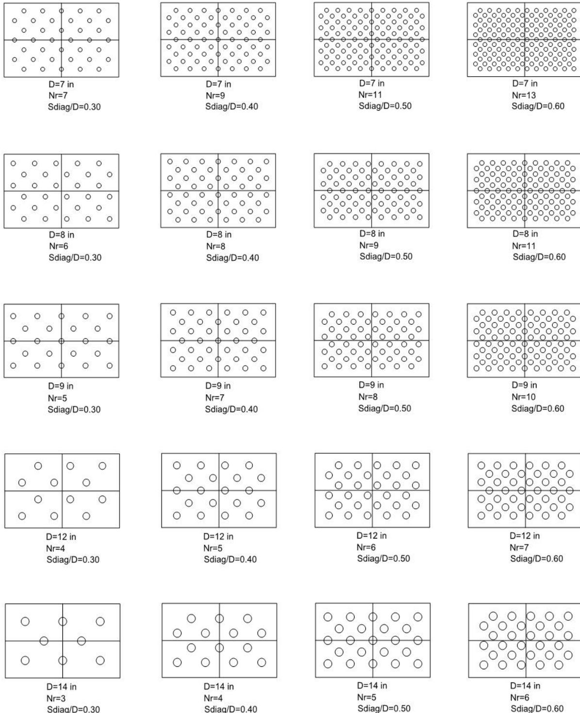
Fig. 3 – Relationship between hole patterns and perforation ratios for a typical 225 in by 125 in web plate
