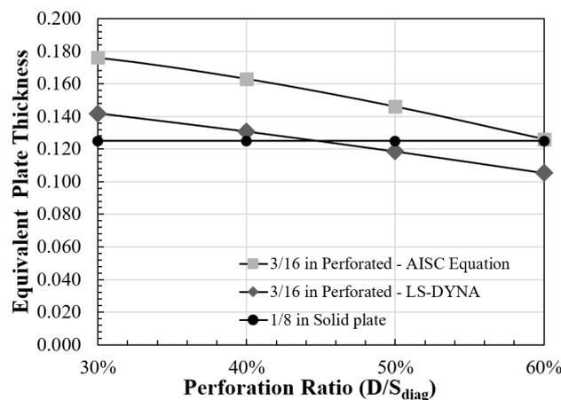
Fig. 10 – Equivalent web plate thicknesses per the AISC 341 equations and LS-DYNA analysis
