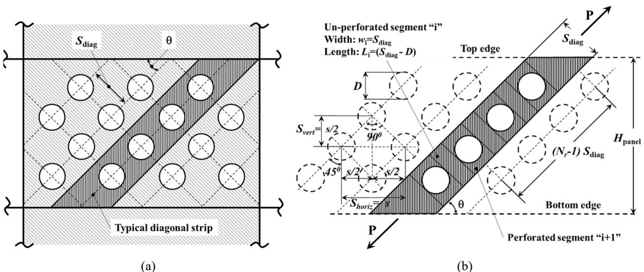
Fig. 1 – Typical hole layout (a) of special perforated SPSW and typical diagonal strip (b) (Vian 2005 [1])
