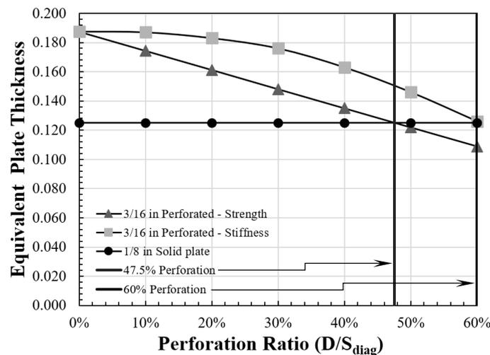
Fig. 2 – Reduction of strength and stiffness of a 3/16" web plate due to perforations.
