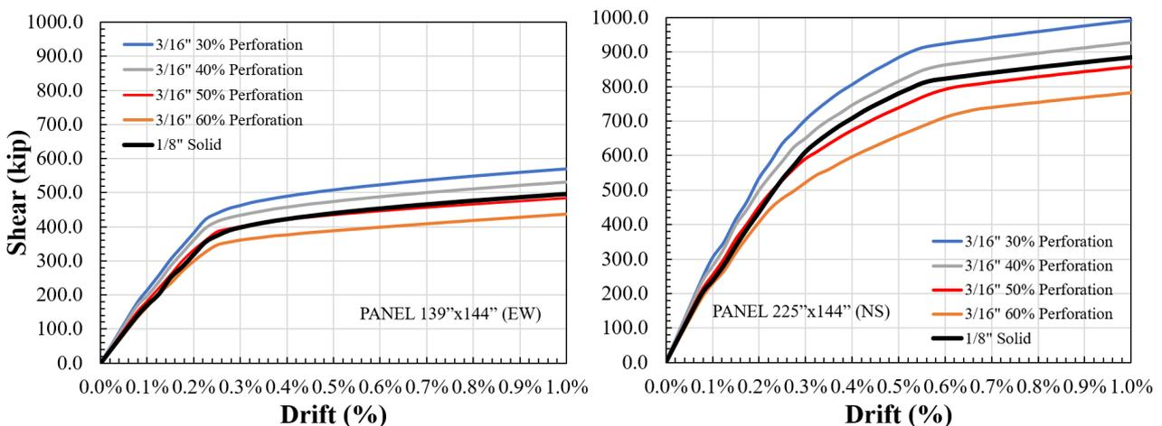
Fig. 7 – Pushover of a single panel with various perforation ratios
