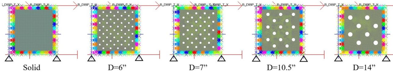
Fig. 8 – LS-DYNA model of a panel with 40% perforation ratio with holes varying from 6” to 14” in diameter
