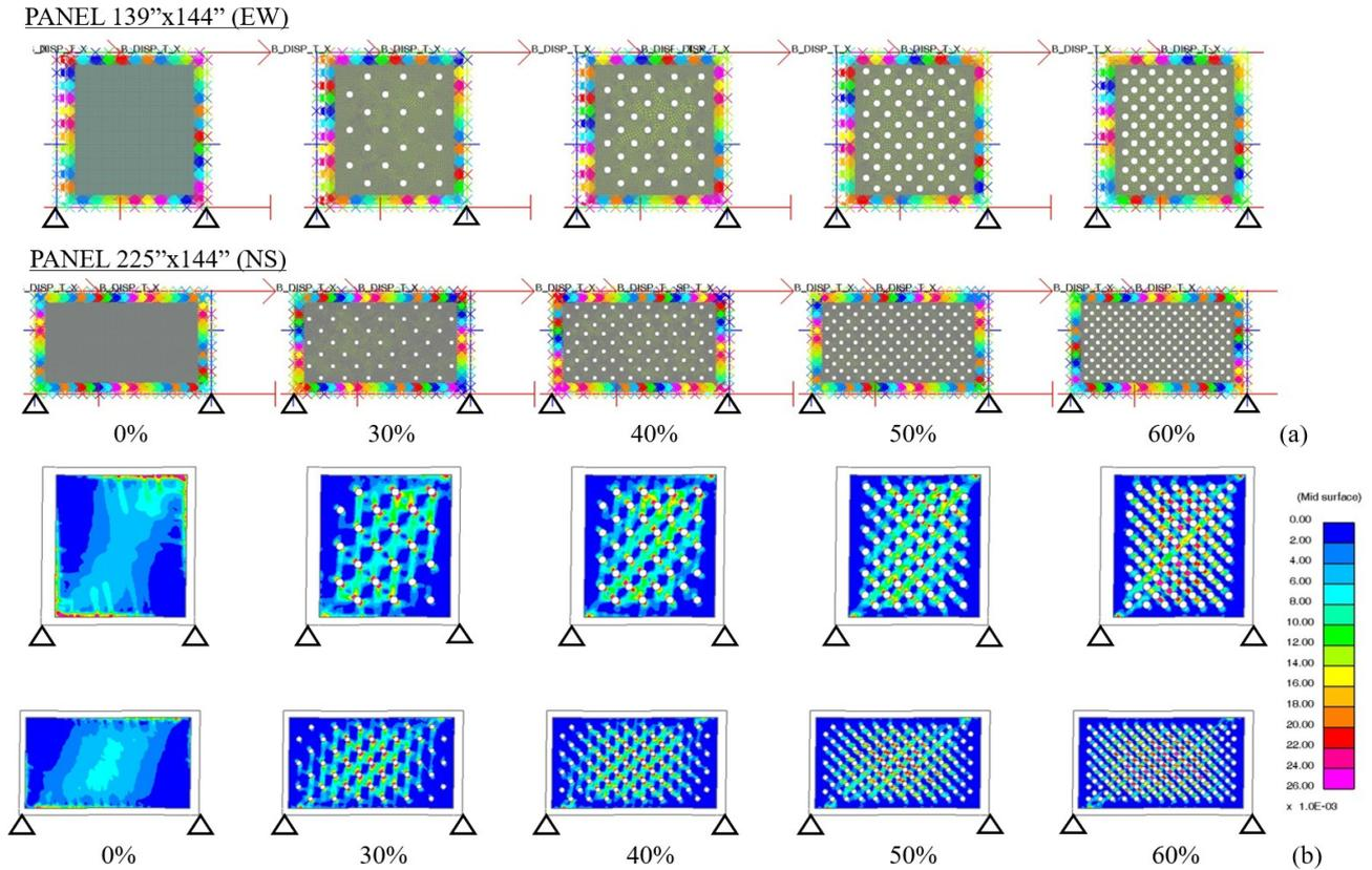
Fig. 6 –LS-DYNA models of two panels with increasing quantity of 7in (hole dia) perforations. Geometry above, strain distribution below.
