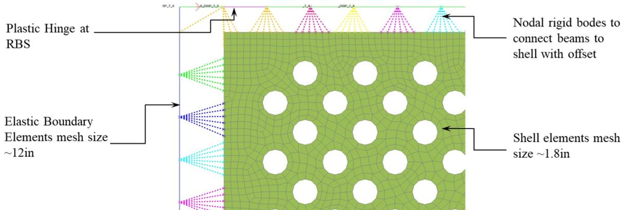
Fig. 4 – Quarter FE model of the perforated SPSW capturing both yielding and buckling of the members.
