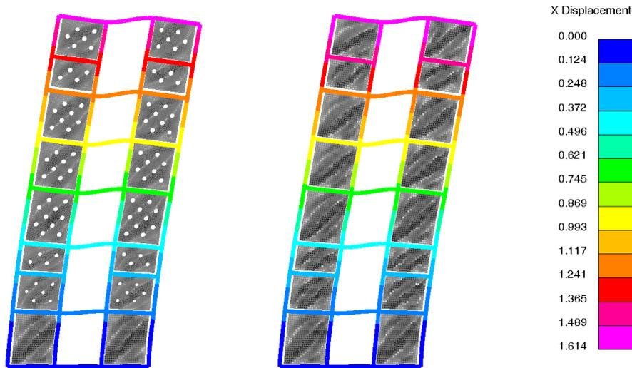
Fig. 14 – Wall displacement (100x magnified) at MCE demands – perforated SPSW (proposed, left) and solid SPSW (original, right).
