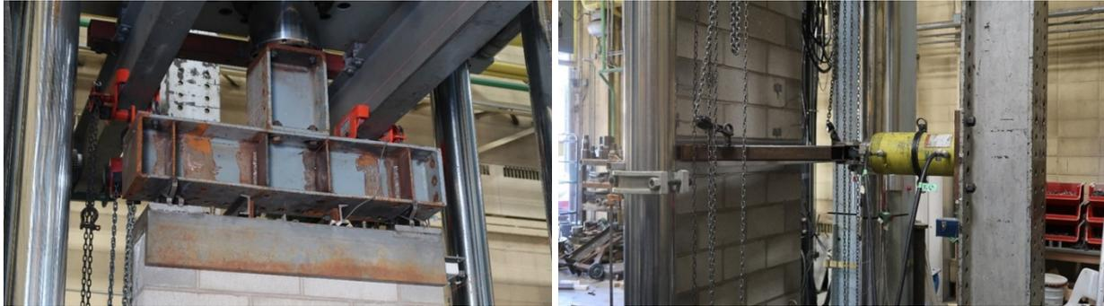
Fig. 5 – a) Gravity Load Application b) Lateral Load Application
