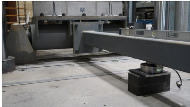
Fig. 6 – Simulation of the Base Rotational Stiffness
