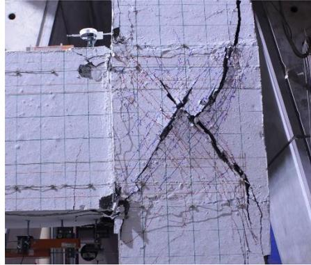
Fig. 7 – Final failure and crack patterns of LAHHV\_SF
