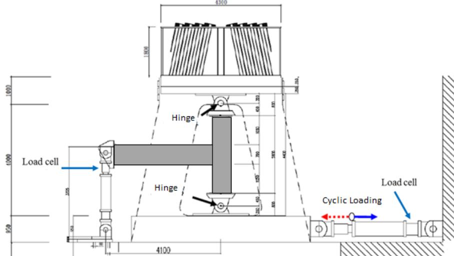
Fig. 2 – Test setup with MATS
