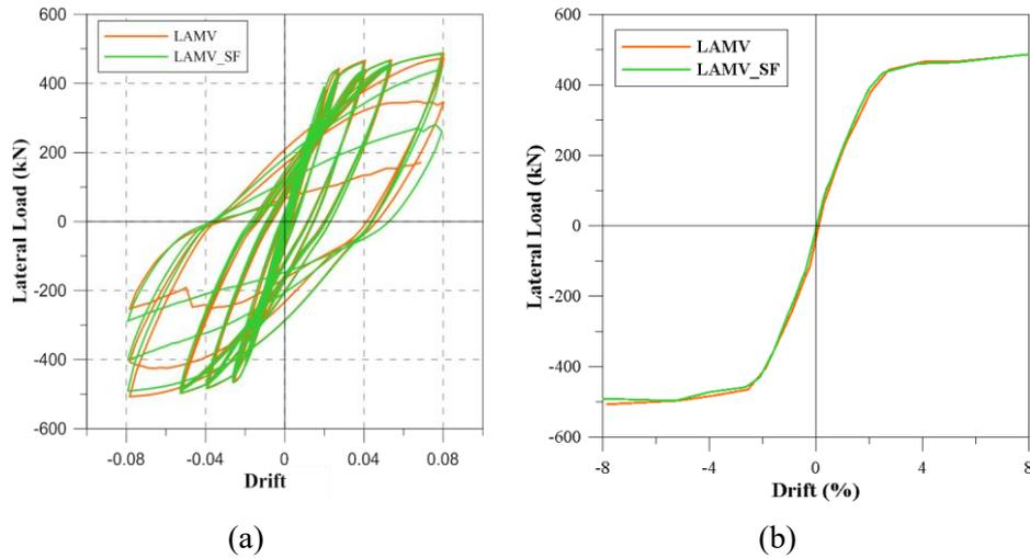
Fig. 4 – (a) Hysteresis loops; (b) hysteresis loop envelopes of LAMV and LAMV\_SF
