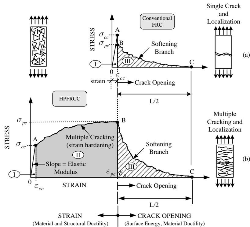
Fig. 1 – Stress-strain response of conventional FRC and HPRC [1]
