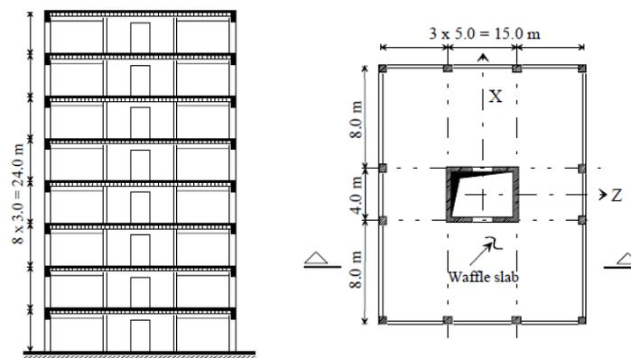
Fig. 1 – Target structure in elevation (*left*) and in plan (*right*)
