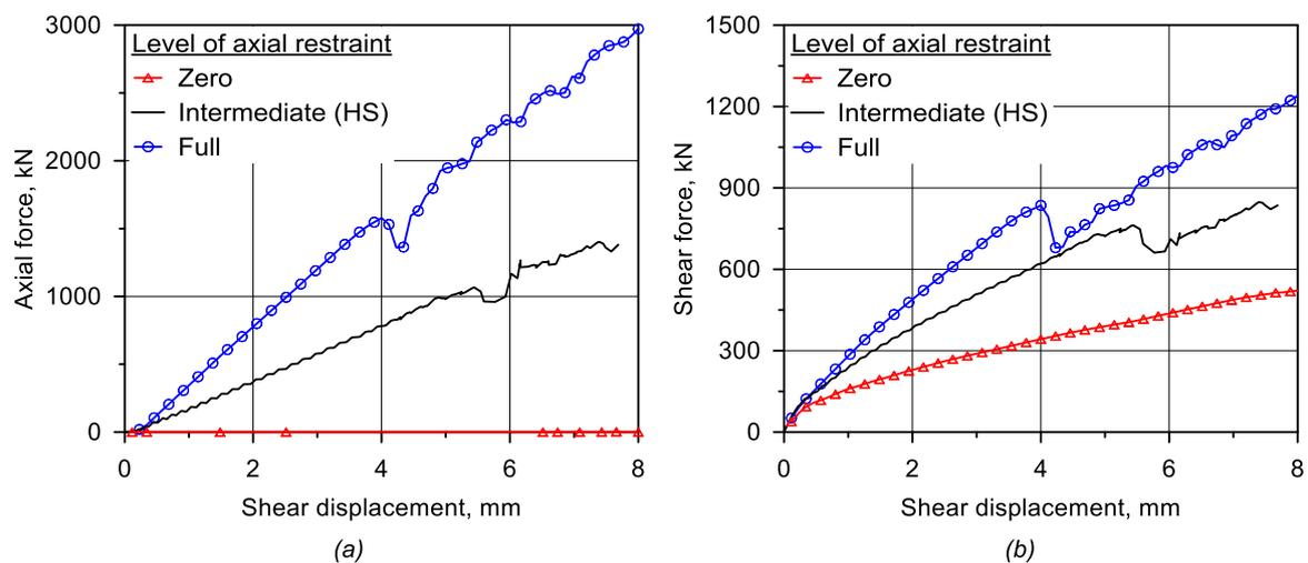
Fig. 8 – Comparison of axial and shear force of coupling beam on 2<sup>nd</sup> floor depending on the level of axial restraint: (a) axial force, (b) shear force
