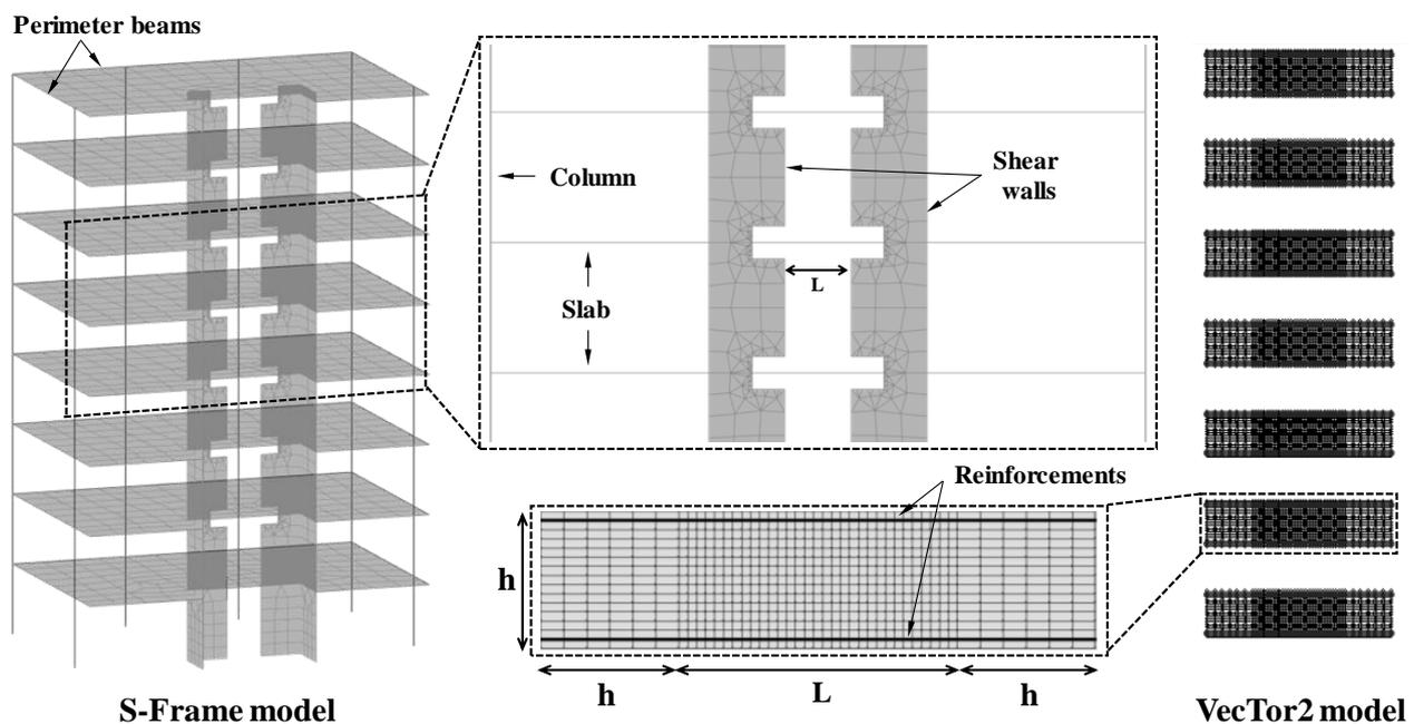
Fig. 2 – Interface node arrangement and meshing
