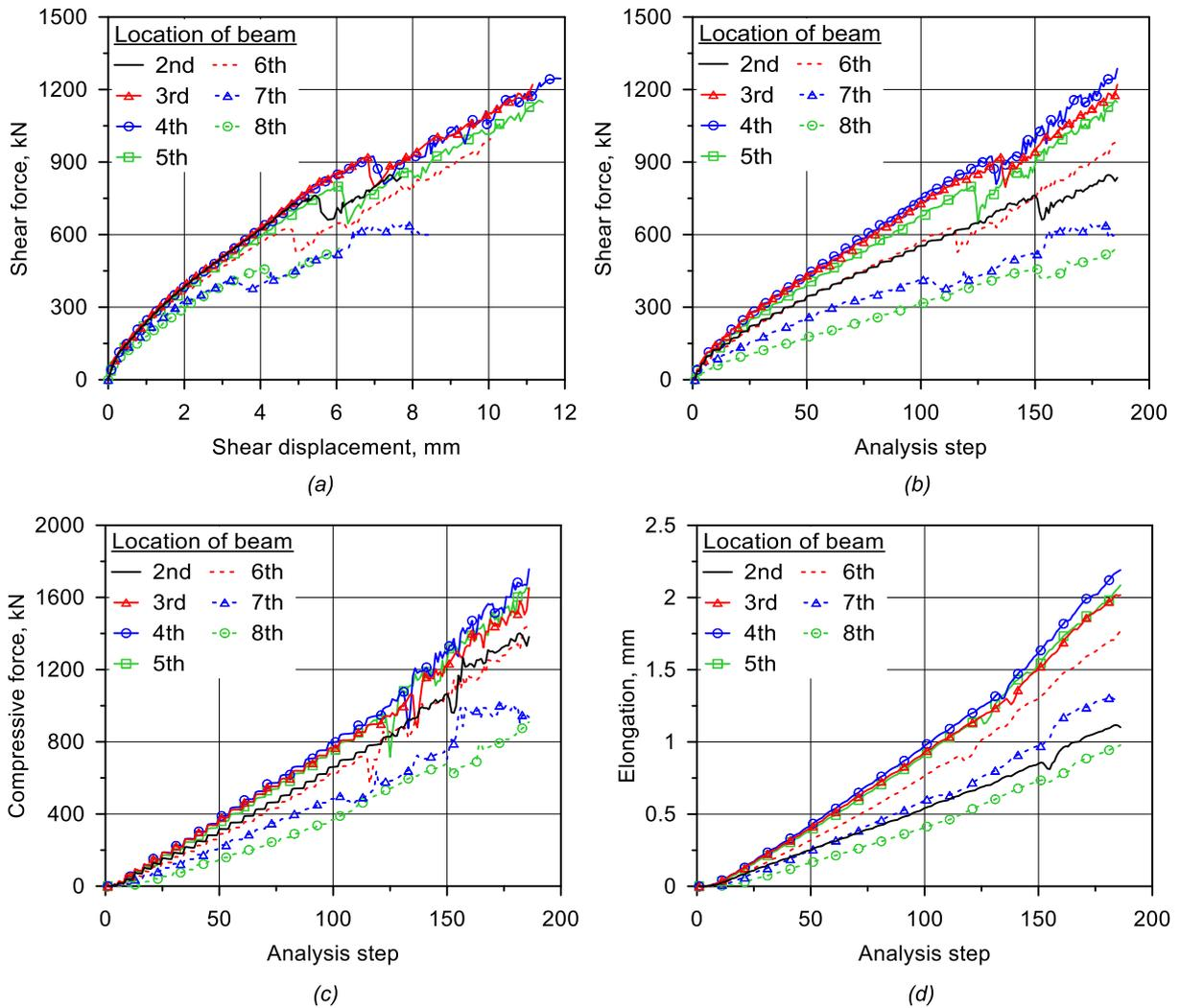
Fig. 5 – Analysis results: (a) shear force-displacement relations, (b) variation of shear force, (c) variation of compressive force, (d) variation of net elongation of beam
