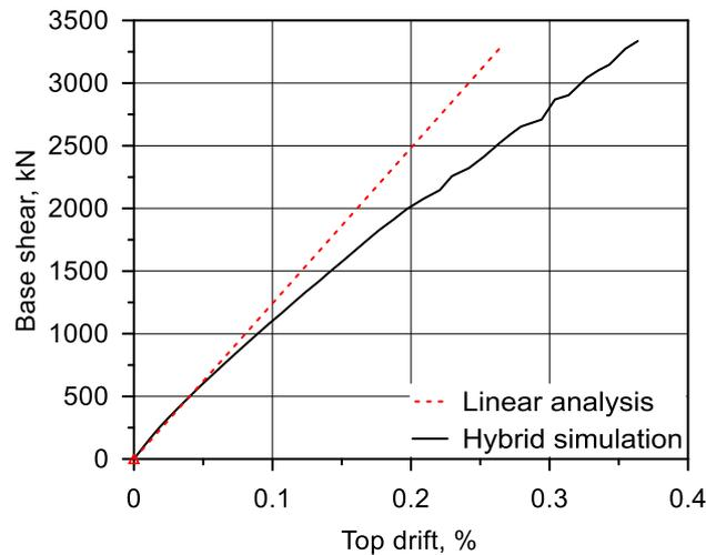
Fig. 7 – Relationship between base shear and top drift
