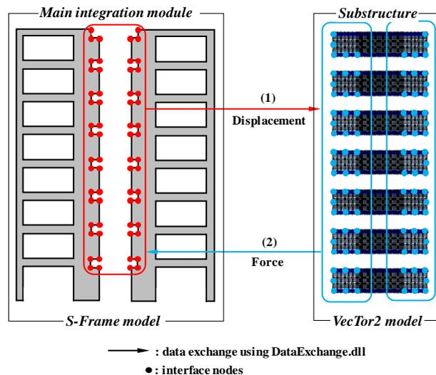
Fig. 4 – Communication between the two numerical model during hybrid simulation
