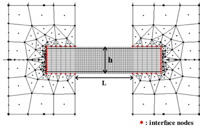
Fig. 3 – Interface node arrangement
