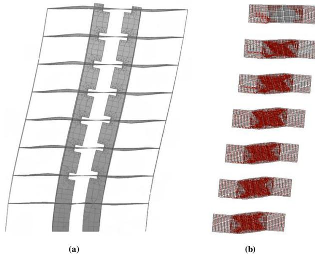
Fig. 6 – Deformation of numerical models in S-Frame and VecTor2: (a) S-Frame model, (b) Coupling beams in VecTor2 model
