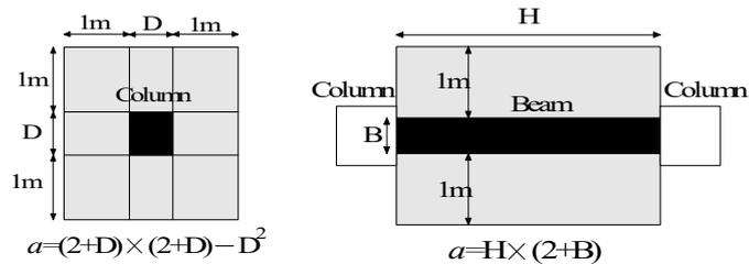
Fig. 2 – Repair work areas of column and beam
