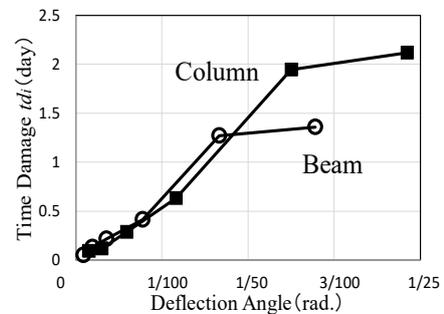
Fig. 8 – Evaluation of time damage for beam and column
