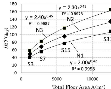
Fig. 10 – Increase in IRT with total floor area
