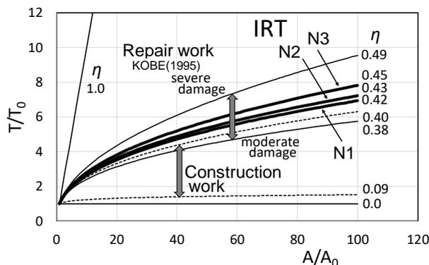
Fig. 9 – Relative increase in repair time with total floor area
