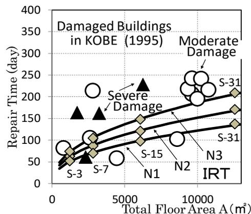
Fig. 11 – Repair time in KOBE earthquake (1995) and IRT
