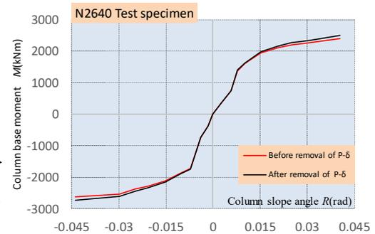
Fig.24 approximate skeleton curves before and after removal of the  $P-\delta$  effect
