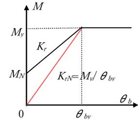
Fig.16 Column base bending stiffness
