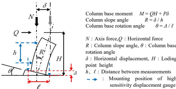
Fig.12 Column slope angle and column base rotation angle
