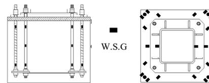
Fig.13 Strain gauge position
