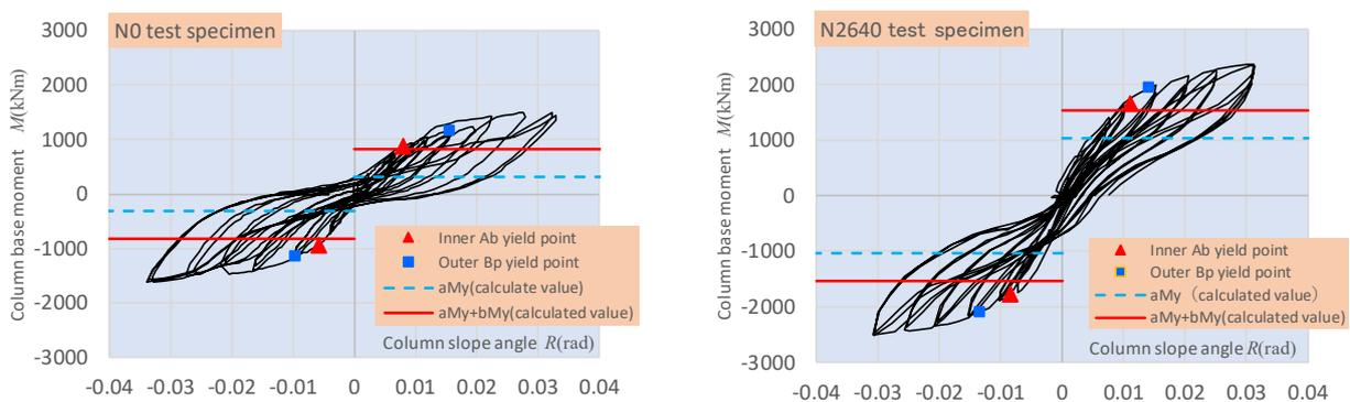
Fig.14 Relationship between column base moment  $M$  and column slope angle  $R$
