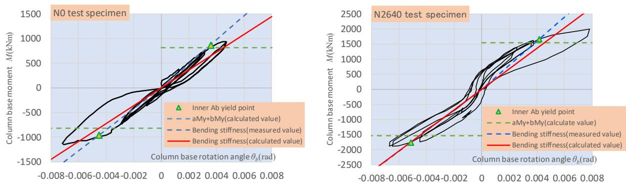
Fig.15 Relationship between column base moment  $M$  and column base rotation angle  $\theta_b$  (till inner  $A_b$  yield cycle)
