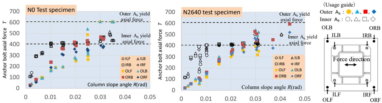
Fig.18 Relationship between anchor bolt acting axial force  $T$  and column slope  $R$
