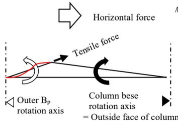
Fig.22 Outer  $B_p$  and column base rotation axis
