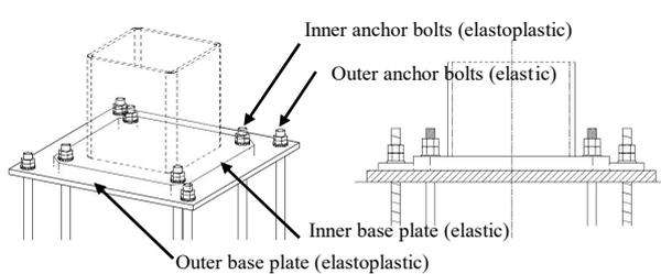
Fig.2 Outline drawing of composite-type exposed column base
