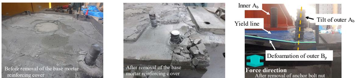
Photo.2 Situation regarding the base mortar and the baseplate after the the test
