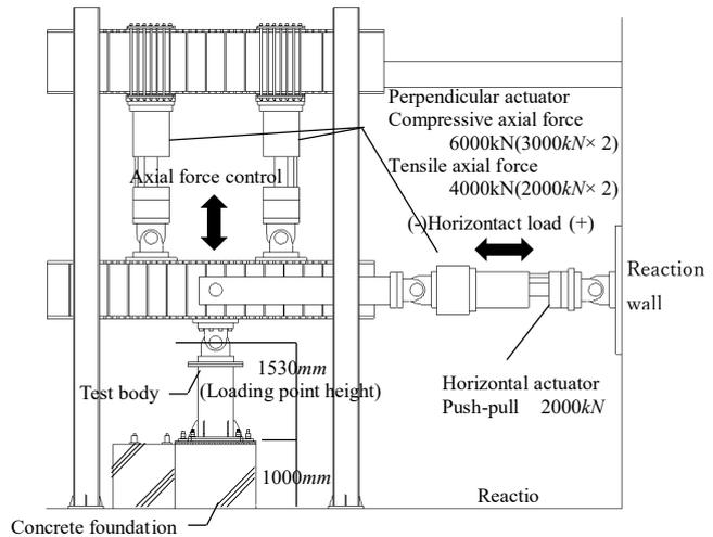
Fig.11 Stress application device
