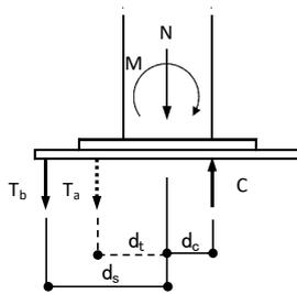
Fig.17 Load-resisting mechanism
