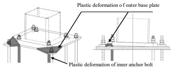
Fig.3 Deformation of composite-type exposed column base during an earthquake
