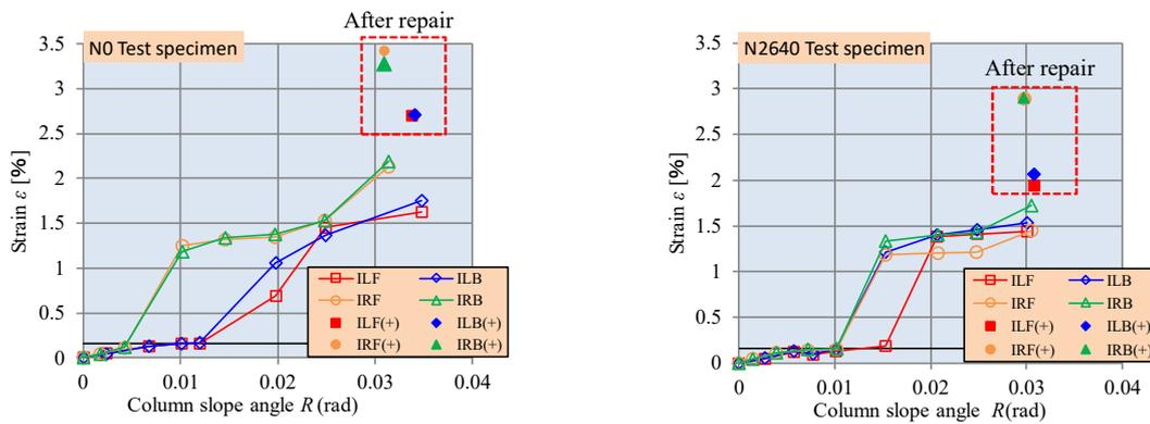
Fig.21 Relationship between  $\varepsilon$  and  $R$  after repair
