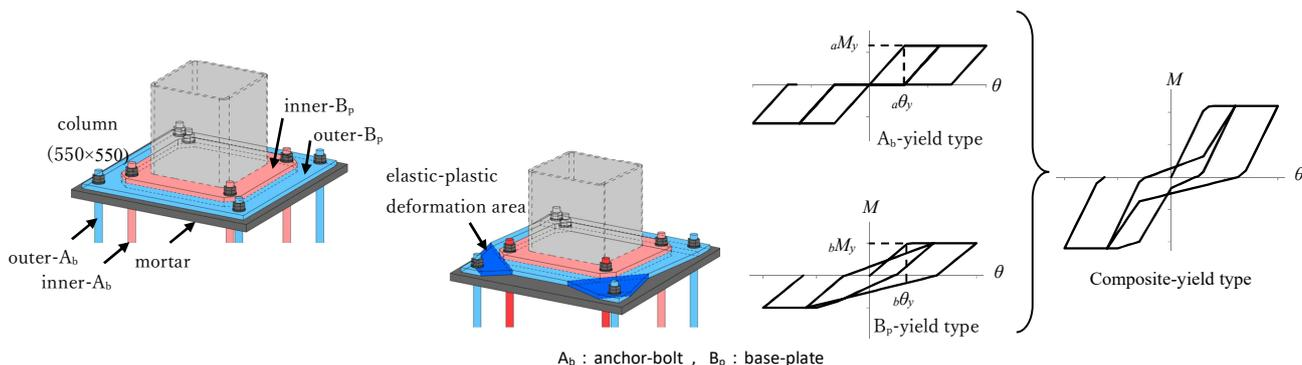
Fig.1 Member configuration of composite-type exposed column base
