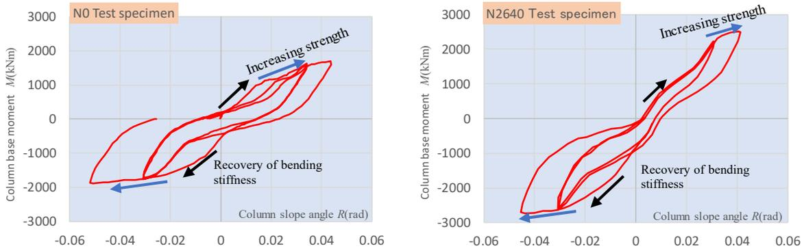
Fig.20 Relationship between  $M$  and  $R$  after repair
