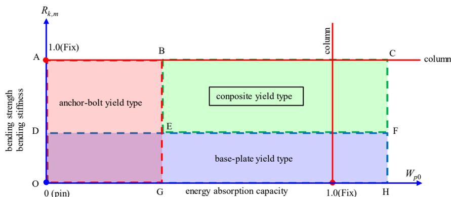
Fig. 1 Conceptual diagram of energy absorption by the exposed type column base
