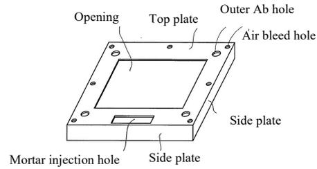
Fig.6 Base mortar reinforcing cover
