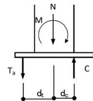
Fig.7 Load resisting mechanism
