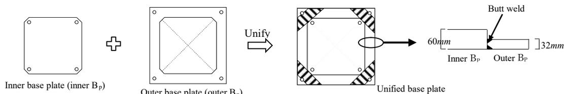
Fig.4 Outline drawing showing manufacture of base plate
