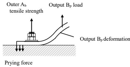
Fig.5 Mechanism of prying force
