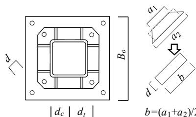
Fig.8 Symbols representing dimensions of each part
