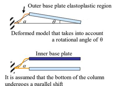
Fig.9 Base plate deformation model
