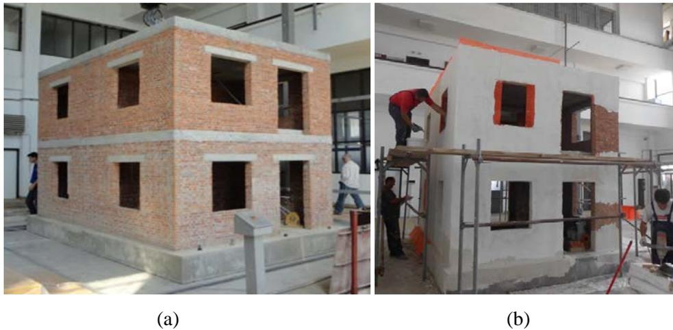
Fig. 3 – Laboratory model – initial state before testing (a); retrofitting process between two tests (b)
