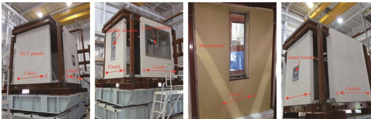
Fig. 2 – The precast cladding system
