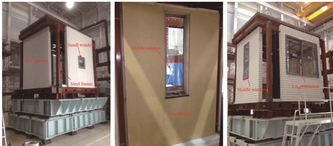
Fig. 2 – The precast cladding system
