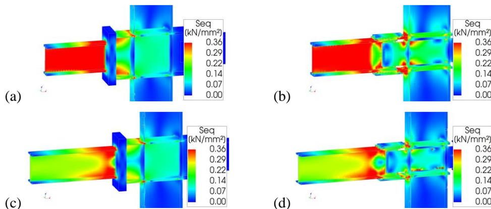
Fig. 13 - von Mises equivalent stresses obtained at link yielding for (a) CC-1.2, (b) CC-2.2, (c) CC-1.6 and (d) CC-2.6 connection
