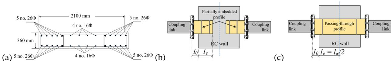
Fig. 3 – (a) Reinforcement detailing for RC wall of the 6-storey HCW system [3] and schematic diagram of (b) WC-1 configuration (c) WC-2 configuration
