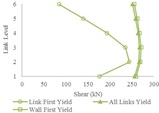
Fig. 7 - Shear in the links for the LRS-HCW with CR 60% and uniform link distribution
