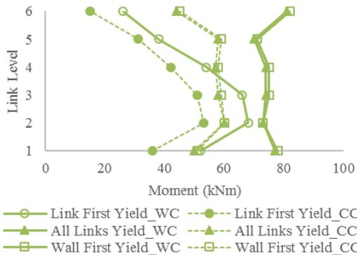
Fig. 9 - Moment in the links for the LRS-HCW with CR 60% and uniform link distribution
