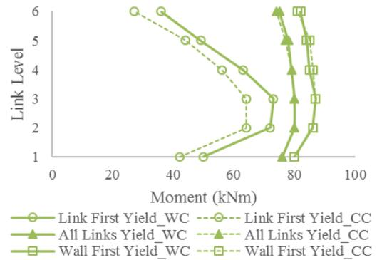
Fig. 10 - Moment in the links for the LRF-HCW with CR 60% and uniform link distribution
