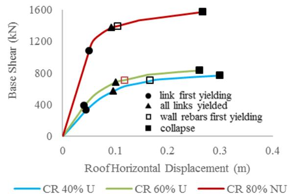
Fig. 6 - Pushover curves for a 6-storey LRF-HCW system
