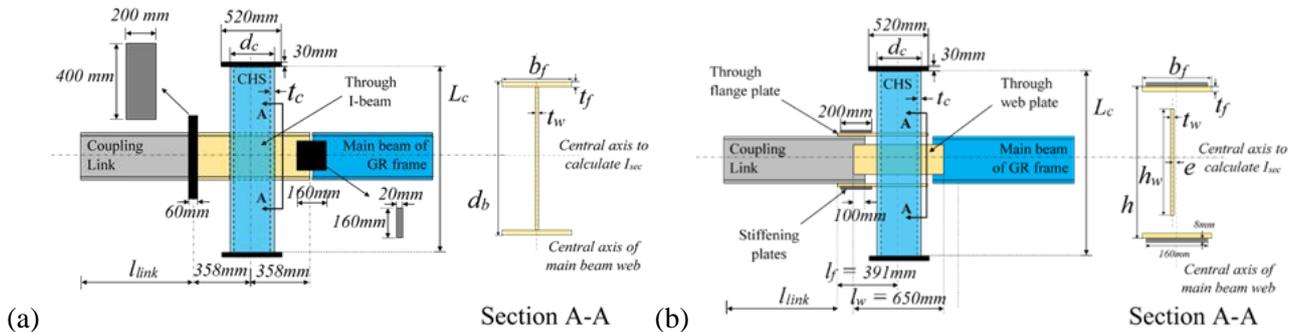
Fig. 4 – Schematic diagram of LASTEICON (a) CC-1 configuration and (b) CC-2 configuration
