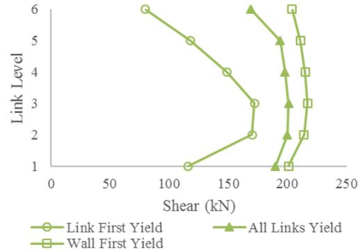
Fig. 8 - Shear in the links for the LRF-HCW with CR 60% and uniform link distribution
