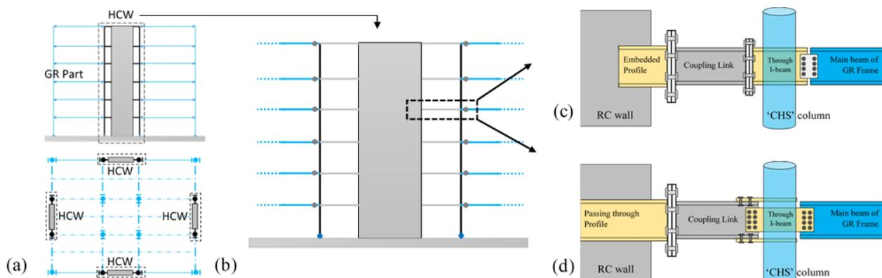
Fig. 1 – (a) Plan view and floor geometry of a 6-storey frame structure with positions of the HCW systems (b) schematic diagram of the HCW system, (c) an example of the “partly embedded” (denoted as WC-1) link-to-wall connection and the “through beam” (denoted as CC-1) link-to-CHS column connection, and (d) an example of the “passing-through” (denoted as WC-2) link-to-wall connection and the “through plates” (denoted as CC-2) link-to-CHS column connection.
