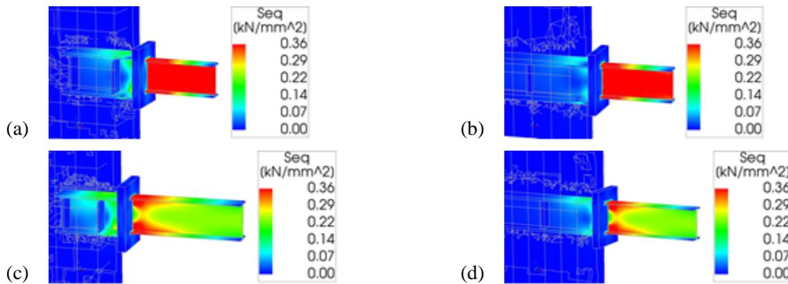
Fig. 11 - von Mises stresses at link yielding for (a) WC\_1.2, (b) WC\_2.2, (c) WC\_1.6 and (d) WC\_2.6
