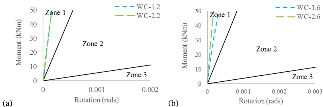
Fig. 12 - Joint classification for (a) WC\_1.2 and WC\_2.2, (b) WC\_1.6 and WC\_2.6
