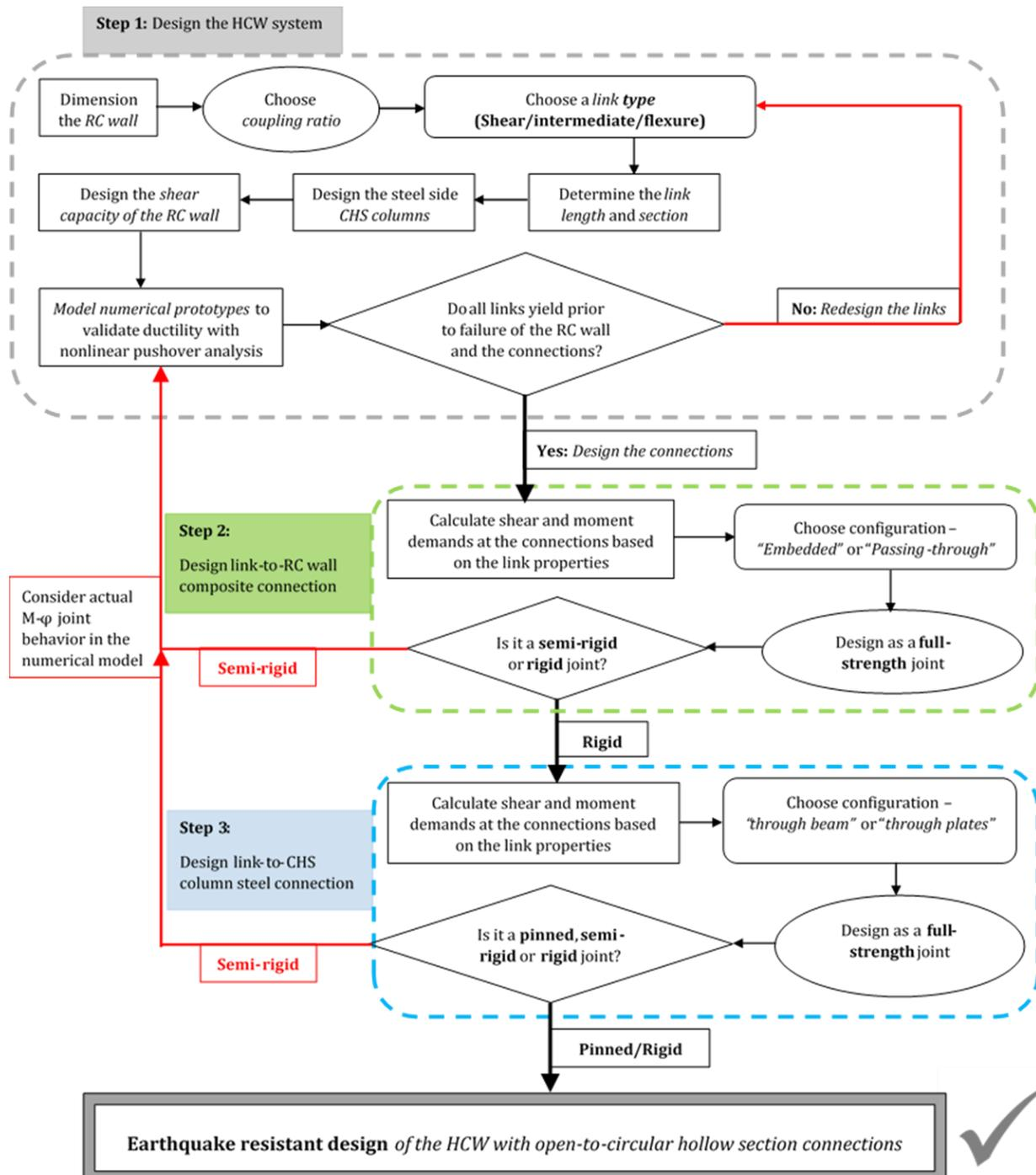
Fig. 2 – General framework for earthquake resistant design of the HCW system with laser-cut open-to-CHS connections
