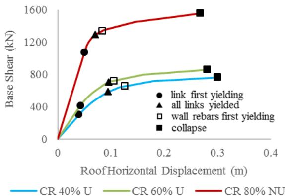
Fig. 5 - Pushover curves for a 6-storey LRS-HCW system
