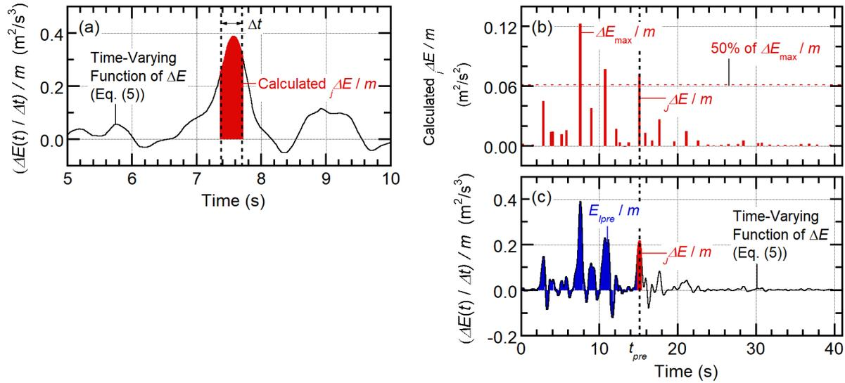
Fig. 2 – Calculation of  $n\Delta E$  and  $E_{Ippe}$  from time-varying function of  $\Delta E$ : (a) calculation of  $n\Delta E$  per unit mass; (b) time history of  $n\Delta E$  per unit mass; (c) calculation of  $E_{Ippe}$  per unit mass.
