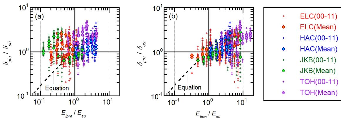
Fig. 8 – Relationship of  $\delta_{pre}/\delta_{su}$  (obtained from time history analysis) and  $E_{Ipre}/E_{su}$  calculated from the time-varying function of  $\Delta E$ : (a) Case A (Eq. (14)); (b) Case B (Eq. (13)).
