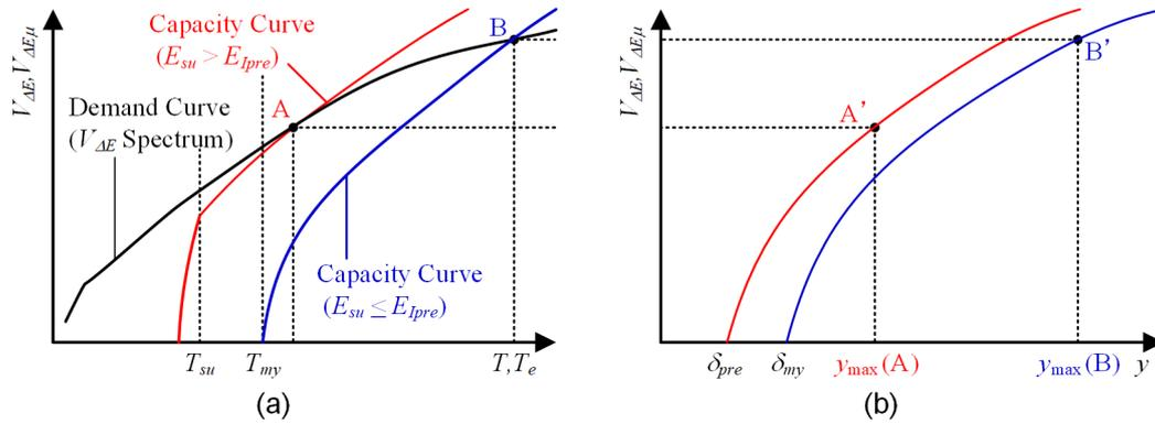
Fig. 4 – Prediction of peak displacement using  $V_{AE}$  spectrum.
