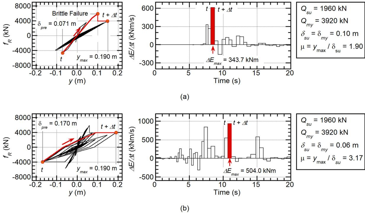
Fig. 1 – Definition of maximum momentary input energy. (a) Model: Cf04Cs02-H15, input ground motion: JKB-00 ( $\alpha_1 = 1.00$ ); (b) model: Cf04Cs02-H09, input ground motion: TOH-00 ( $\alpha_1 = 0.85$ ).
