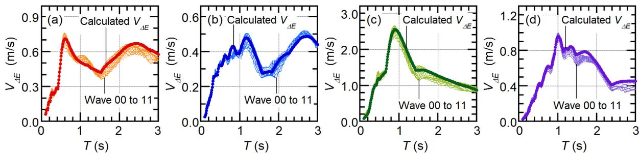
Fig. 6 –  $V_{\Delta E}$  spectrum of unscaled input ground motions: (a) Group ELC; (b) group HAC; (c) group JKB; (d) group TOH.
