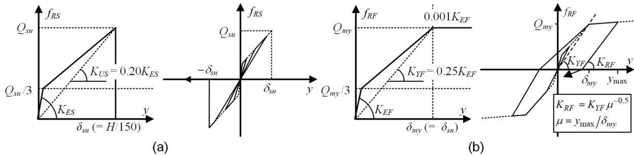
Fig. 5 – Envelopes and hysteresis rules for brittle and ductile RC members: (a) brittle members (dominated by shear behavior); (b) ductile members (dominated by flexural behavior).
