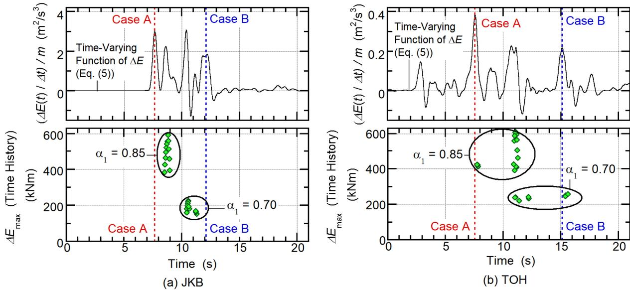
Fig. 9 – Comparisons of  $t_{pre}$  predicted from unscaled time-varying function of  $\Delta E$  and time at  $\Delta E_{max}$  in time history analysis for model Cf04Cs02-H09: (a) JKB group; (b) TOH group.
