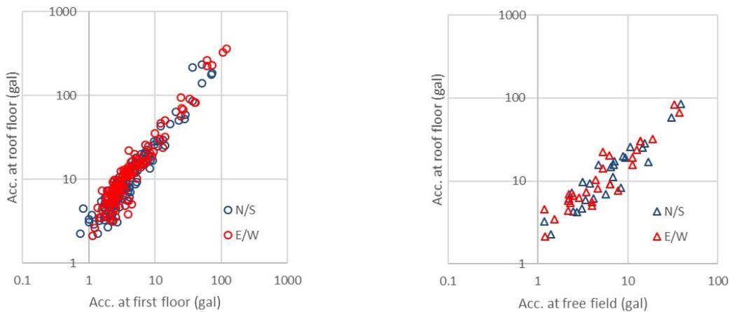
Fig. 3 – Roof level and first floor / free field maximum acceleration
