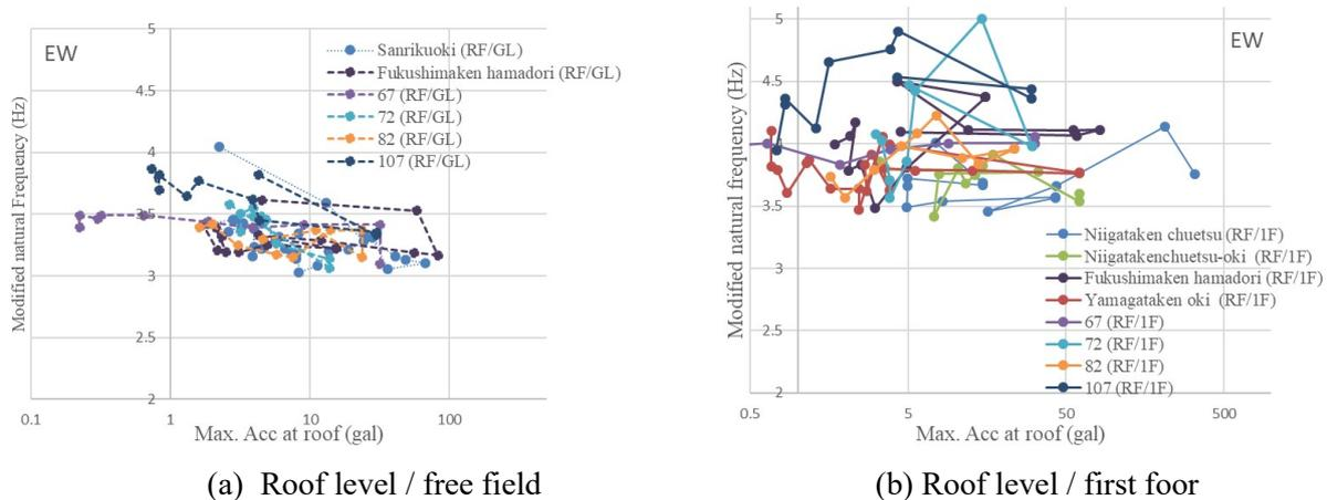
Fig. 8 – Relation of natural frequency to maximum acceleration based on running spectra
