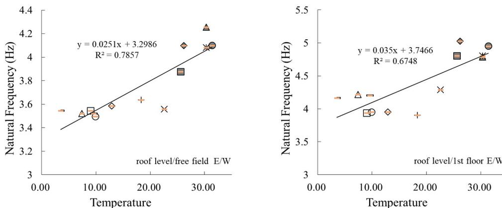
Fig. 5 – Relation of natural frequency of E/W direction to temperature by microtremor measurement [3]
