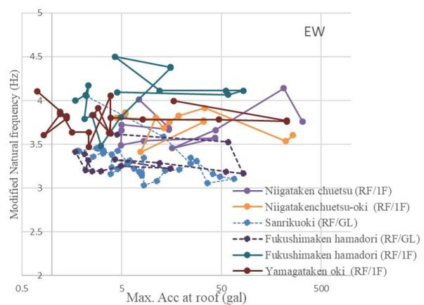
Fig. 7 – Relation of natural frequency to maximum acceleration using running spectra
