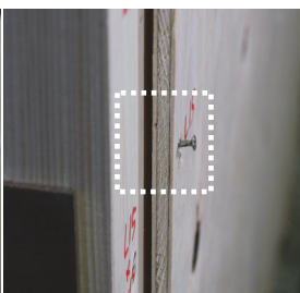
(a) Punching out (b) Bending fracture (c) Pullout
