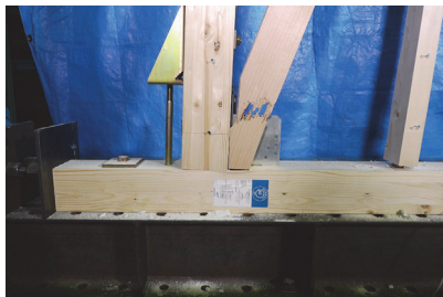
(a) Tensile fracture of brace connection (b) Crack of gypsum board
