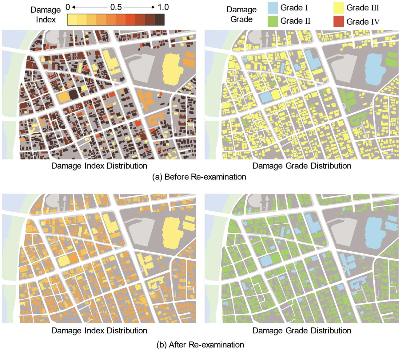
Fig.13 – Estimated seismic damage using the damage spectrum
