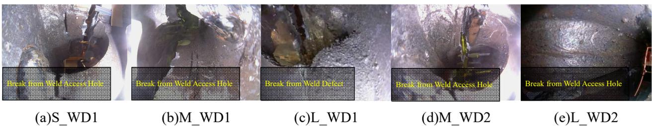
Fig.12 Ultimate state of fracture section of each specimen
