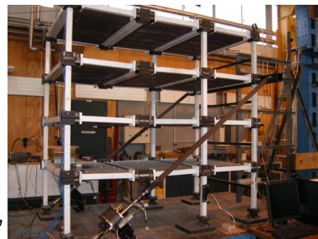
Fig. 6 – Schematic and test model of four-story structure
