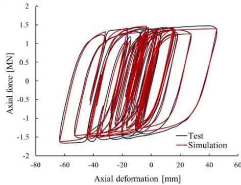
Fig. 3 – Calibration verification using seismic signal (S7 specimen)
