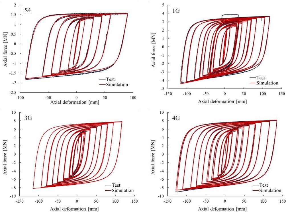
Fig. 2 – BRB Steel4 model calibration
