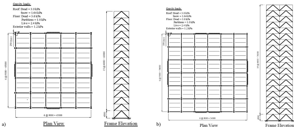
Fig. 4 – Prototype building layouts for: a) 16-storey building; b) 20-storey building
