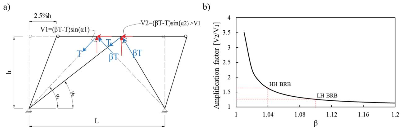
Fig. 14 – Effect of geometrical nonlinearity. a) Beam force demands; b) Amplification factor variation with  $\beta$
