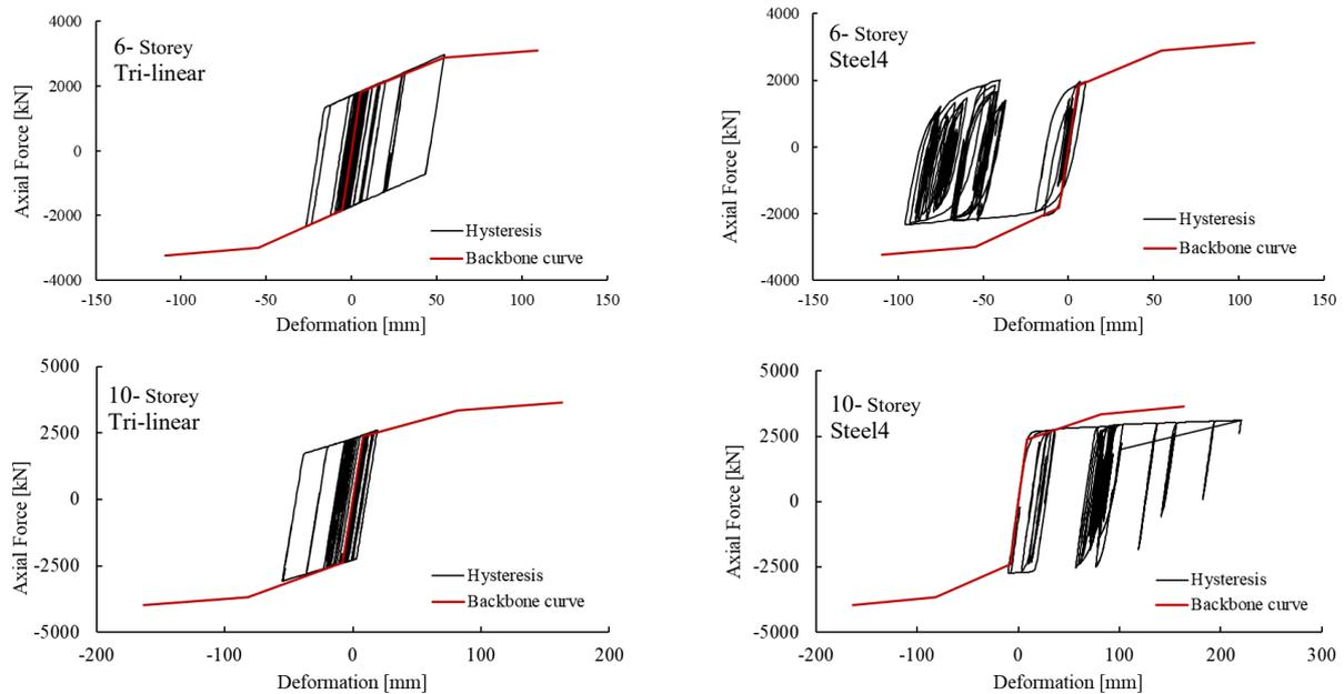
Fig. 10 – BRB hysteresis under subduction interface earthquake
