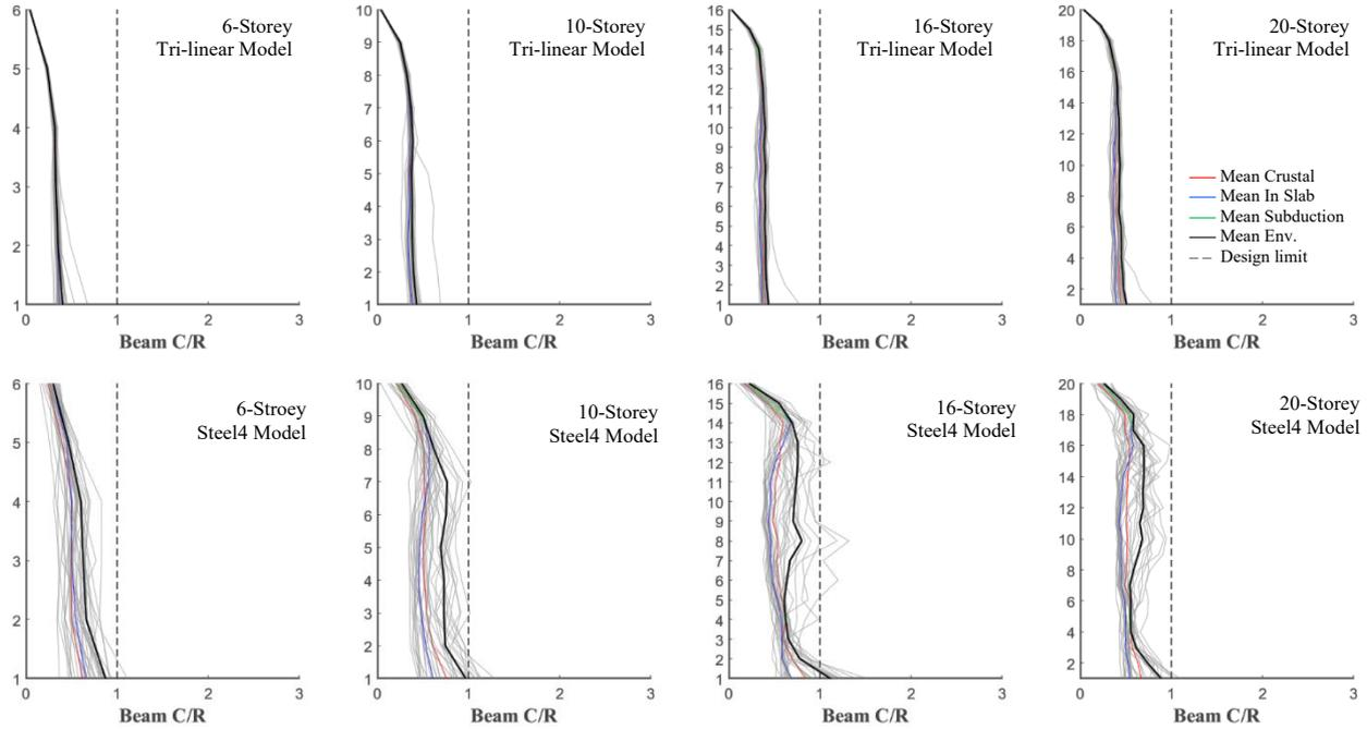
Fig. 12 – Beam demand/design capacity ratio (HH BRBs)
