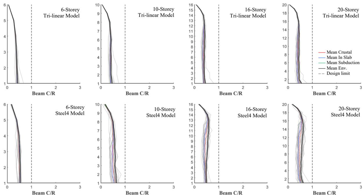
Fig. 11 – Beam demand/design capacity ratio (LH BRBs)
