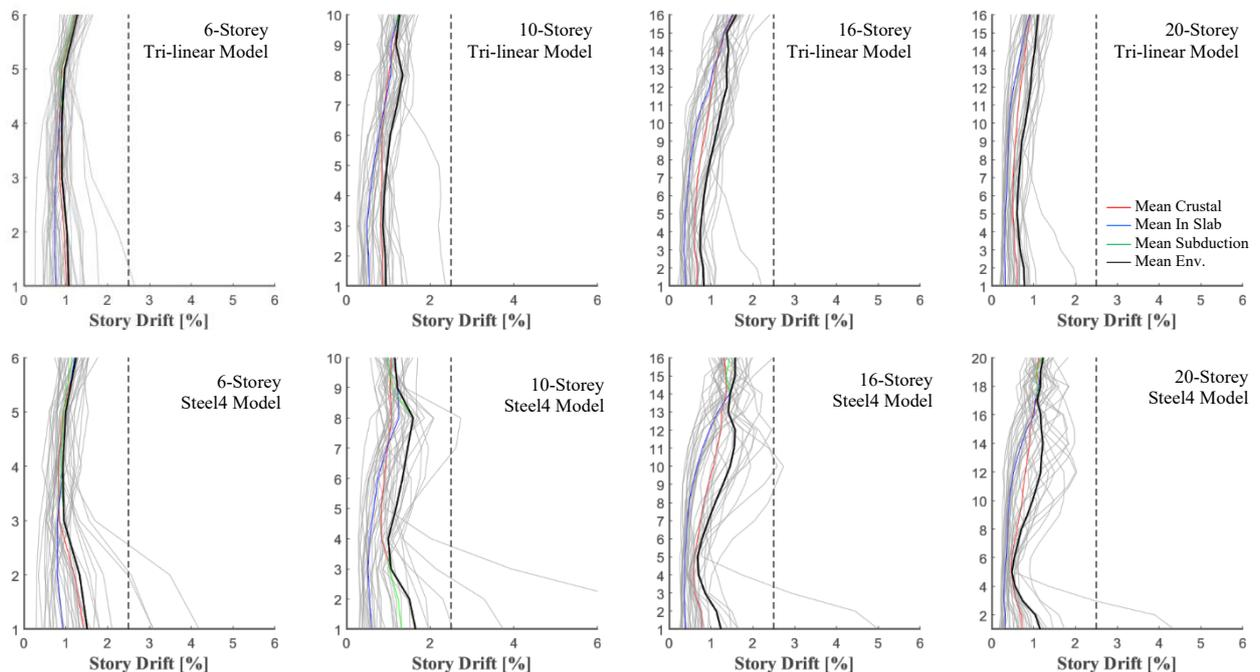
Fig. 9 – Storey drift ratios (HH BRBs)
