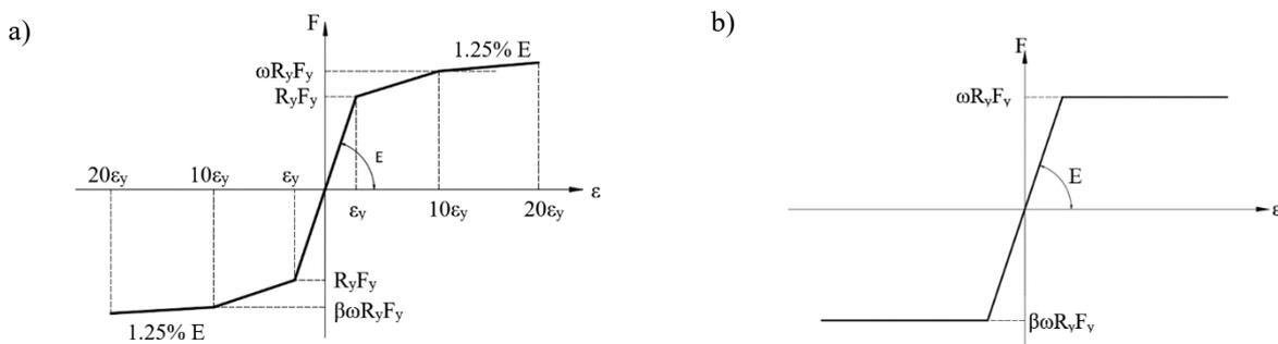
Fig. 1 – Simplified BRB material models. a) Tri-linear BRB model adapted from [5]; b) Bi-linear BRB model
