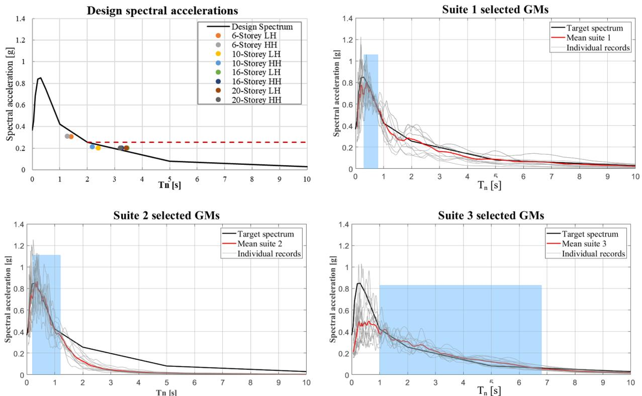
Fig. 5 – Scaled/selected ground motions (Package I)
