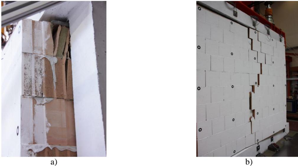
Fig. 4 – a) Damage of the bricks at the top row and b) failure of the BO specimen
