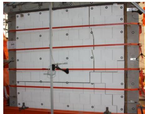
Fig. 8 – a) Top view of the wall deformation in the out-of-plane direction for the horizontal section in the middle height of the wall for different in-plane drifts and b) cracks in the wall at the 1.8% of in-plane drift
