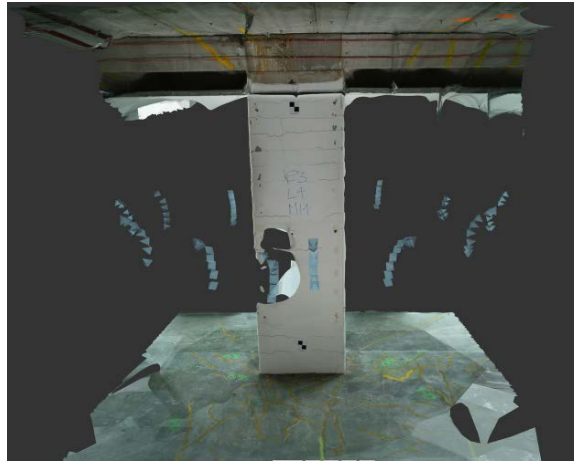
Fig. 6- Showing the poor quality of the model generated with varying light intensities using SFM/MVS
