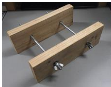
Fig. 7 – Jig for fixing zelkova wood
