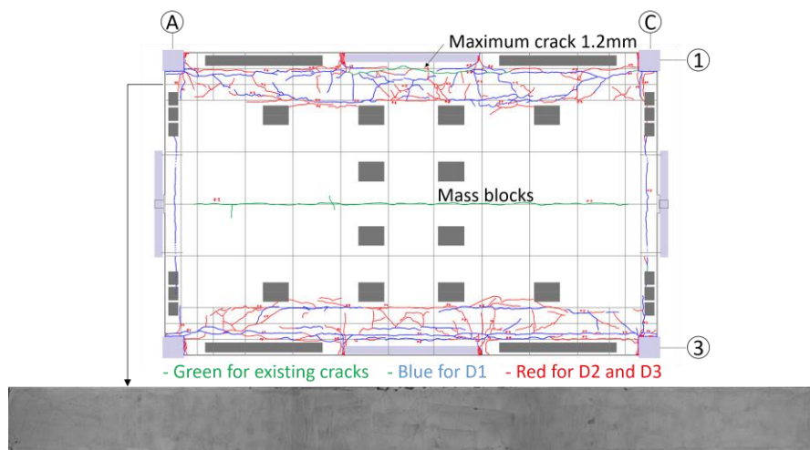
Fig. 16 – Crack map of link slab at end of test
