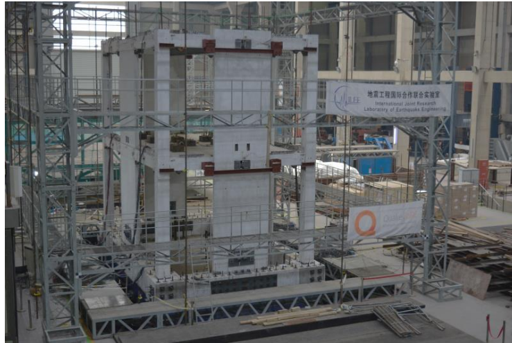
Fig. 1 - The test building on the shake-table array at Tongji University's Jiading campus
