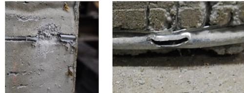
Fig. 9 - Rib around staple after loading
