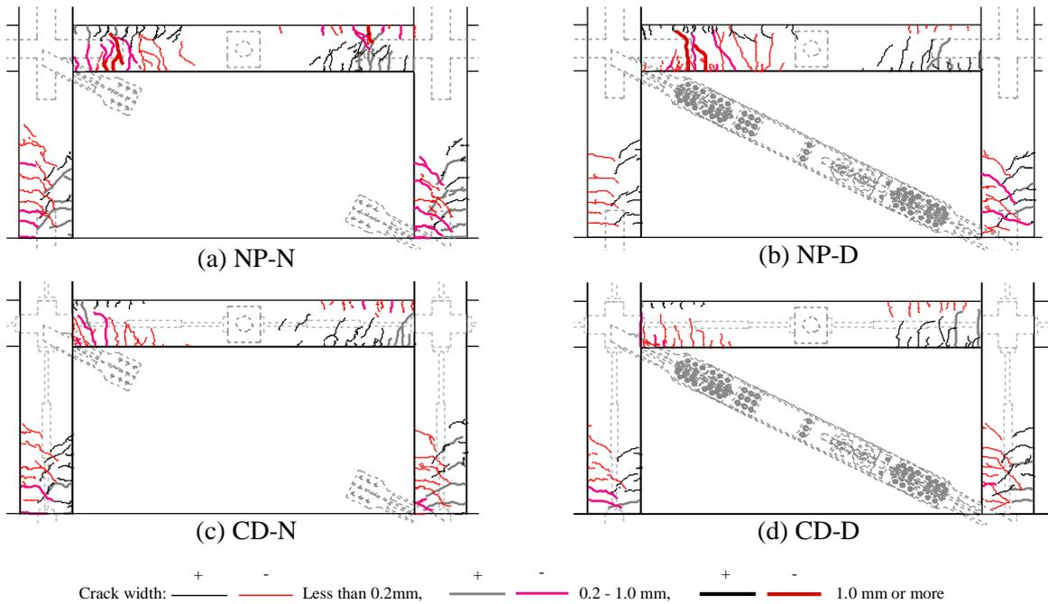
Fig. 5 – Damages of the RC frames at  $R = \pm 1/100$ rad
