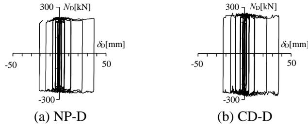
Fig. 6 – Axial force in the damper  $N_D$  versus the sliding displacement of the damper  $\delta_D$  relationship
