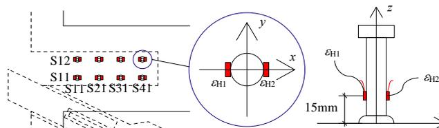
Fig. 11 – Strain gauge sticking position of stud bolts
