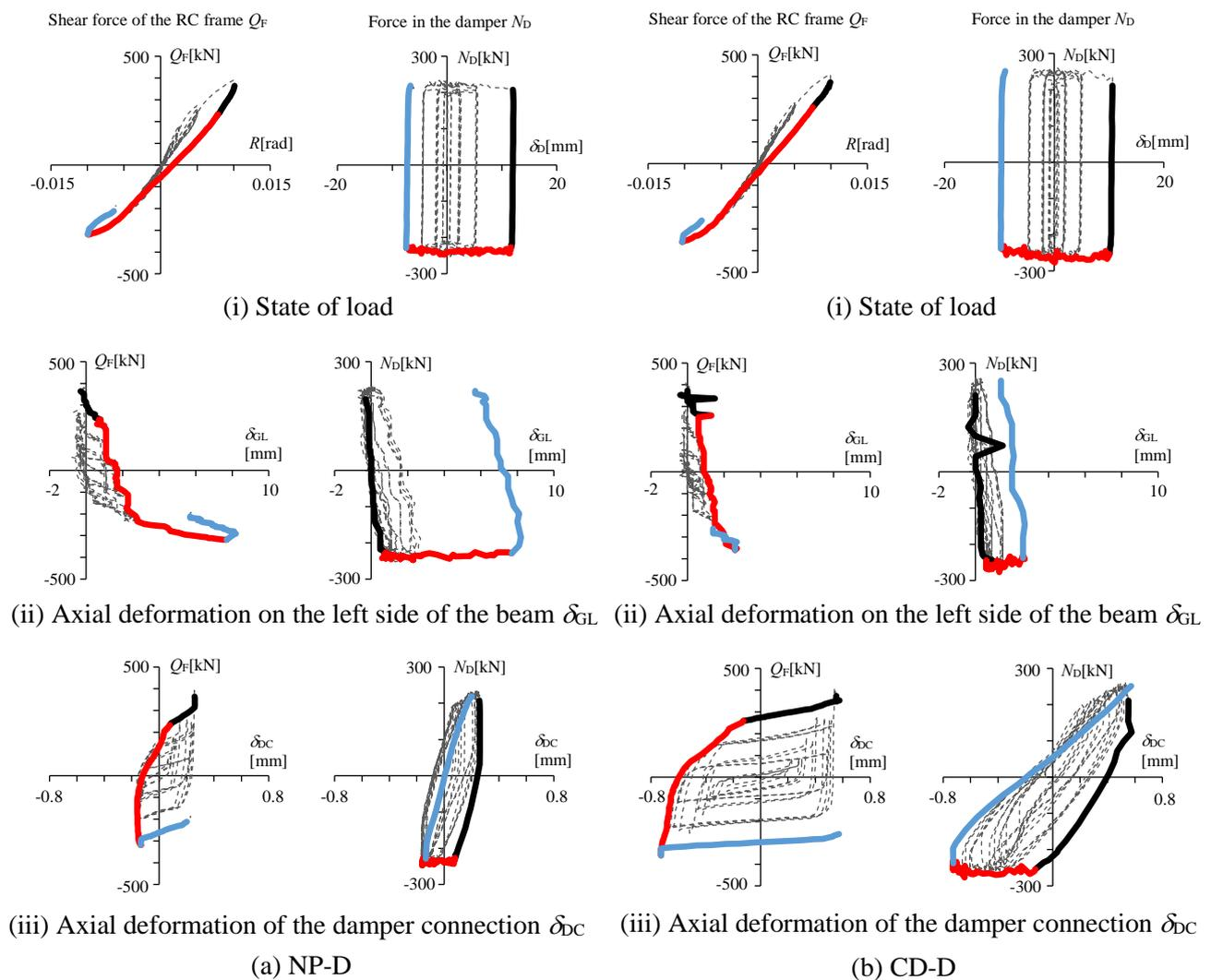
Fig. 10 – Axial deformation of the beam  $\delta_{GL}$  and the axial deformation of the damper connection  $\delta_{DC}$
