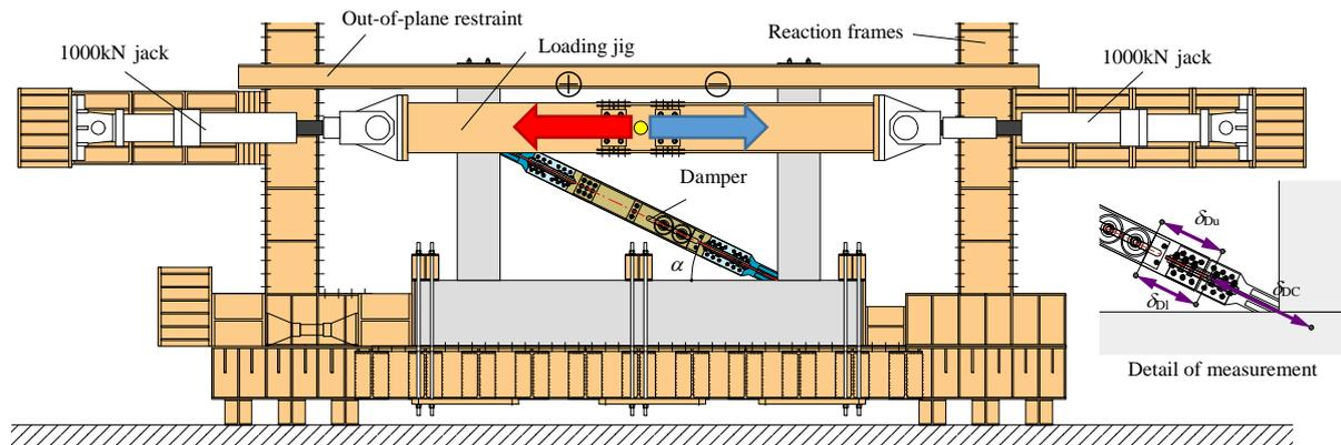
Fig. 3 – Test setup and measurement
