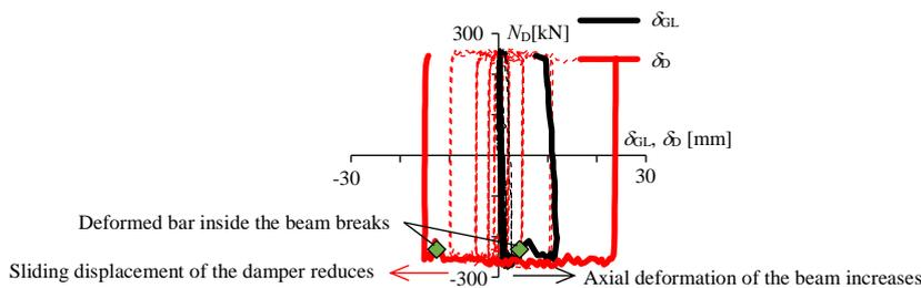
Fig. 9 – Axial deformation of the beam  $\delta_{GL}$  and the sliding displacement of the damper  $\delta_D$
