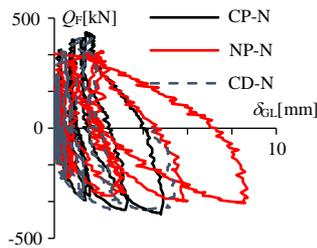
Fig. 8 – Story shear force  $Q_F$  versus the axial deformation on the left side of the beam  $\delta_{GL}$  relationship
