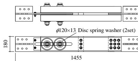
Fig. 2 – Details of damper (Unit: mm)
