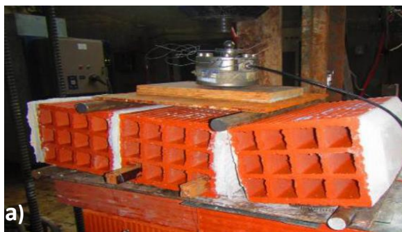
Fig. 13. a) Experimental set up of out of plane triplet bending test b) Flexural stress versus the out of plane displacement obtained by triplet bending tests
