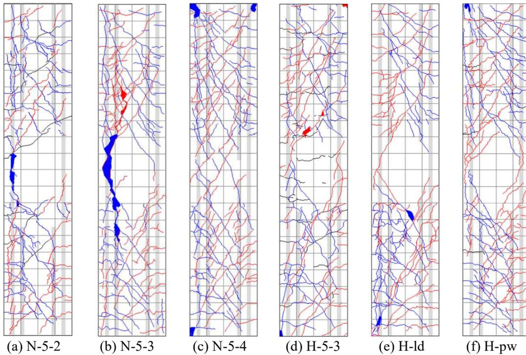
Fig. 8 – Crack Pattern at Peak Load
