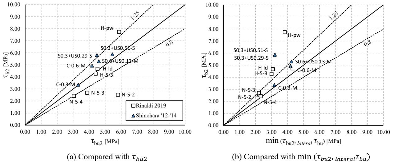
Fig. 6 – Maximum Bond Stress of Second Layer Bars ( $\tau_{b2}$ )
