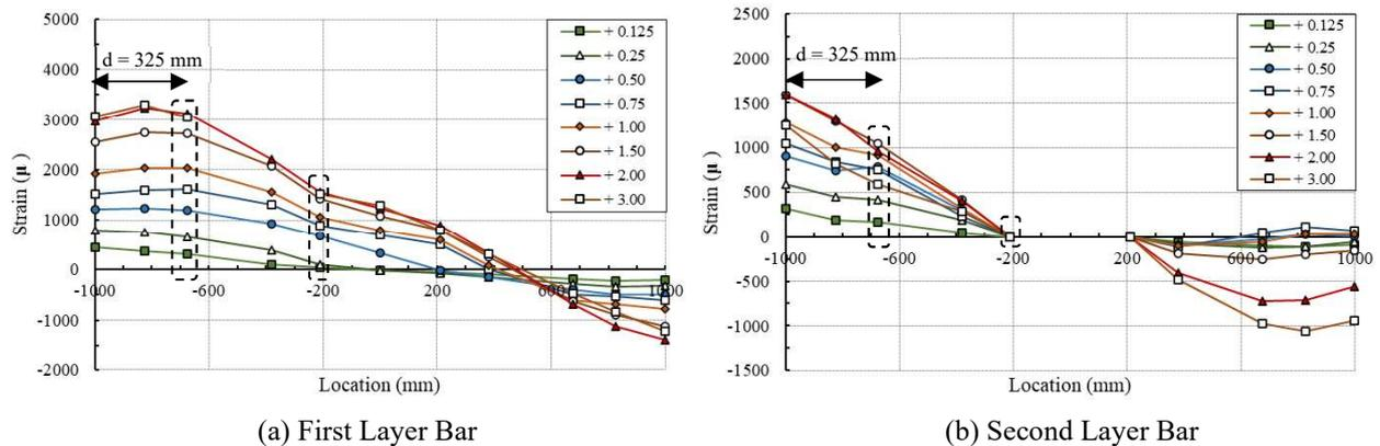
Fig. 5 – Longitudinal Bar Strain Distribution for N-5-3
