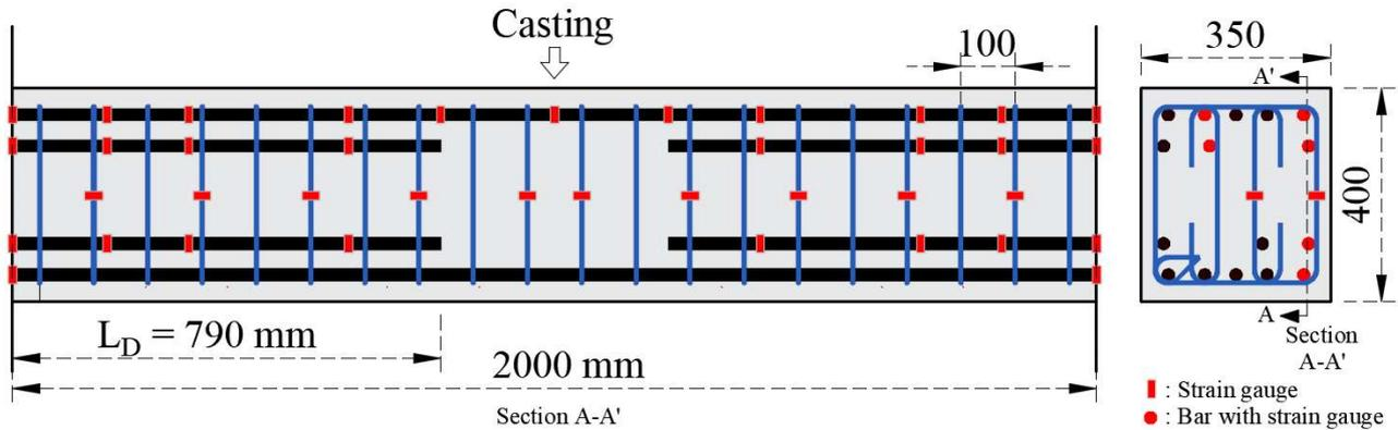
Fig. 4 – Strain Gauges Location for N-5-3
