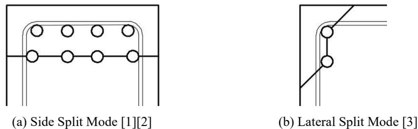
Fig. 1 – Bond Split Failure Modes
