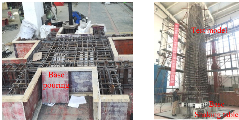
Fig.3 – The model construction process and finished structure
