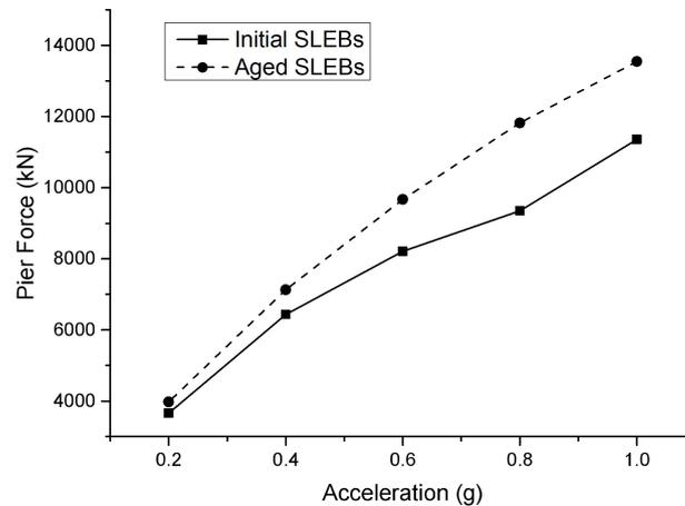
Fig. 11 - Maximum Force of pier bottom section under different level ground motions.
