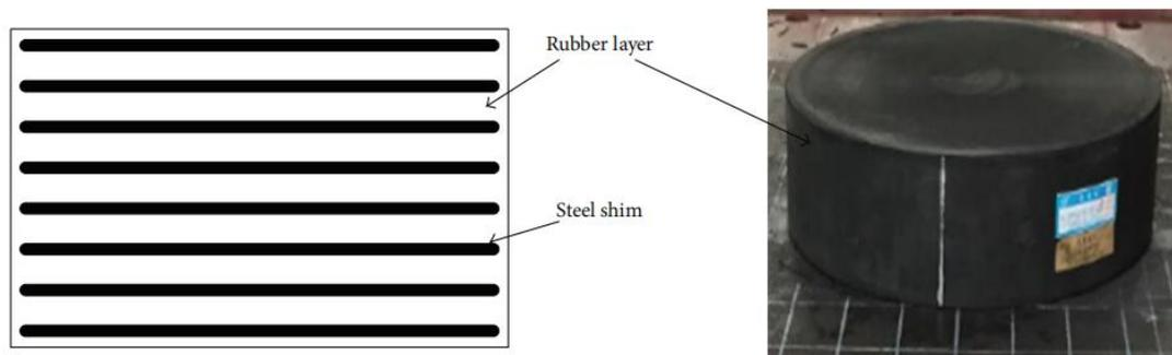
Fig. 2 - Sketch of testing specimens: bearing type Y1/Y2.
