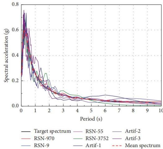
Fig. 9 - Target spectrum and the spectrum of selected ground motions.
