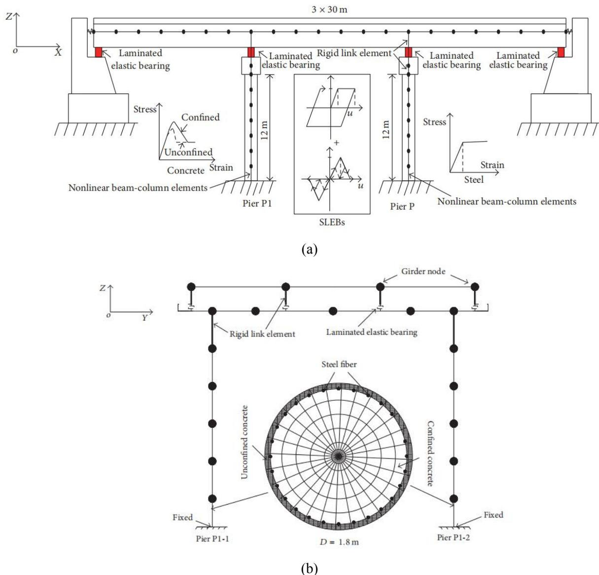
Fig. 8 - Finite element models of the prototype bridge: (a) elevation view; (b) bent elevation at pier P1.
