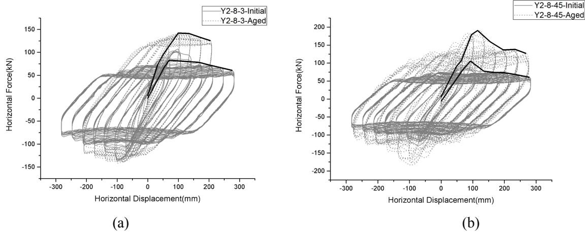
Fig. 4 - Force versus displacement results for the cyclic tests: (a) Y2-8-3; (b) Y2-8-45.
