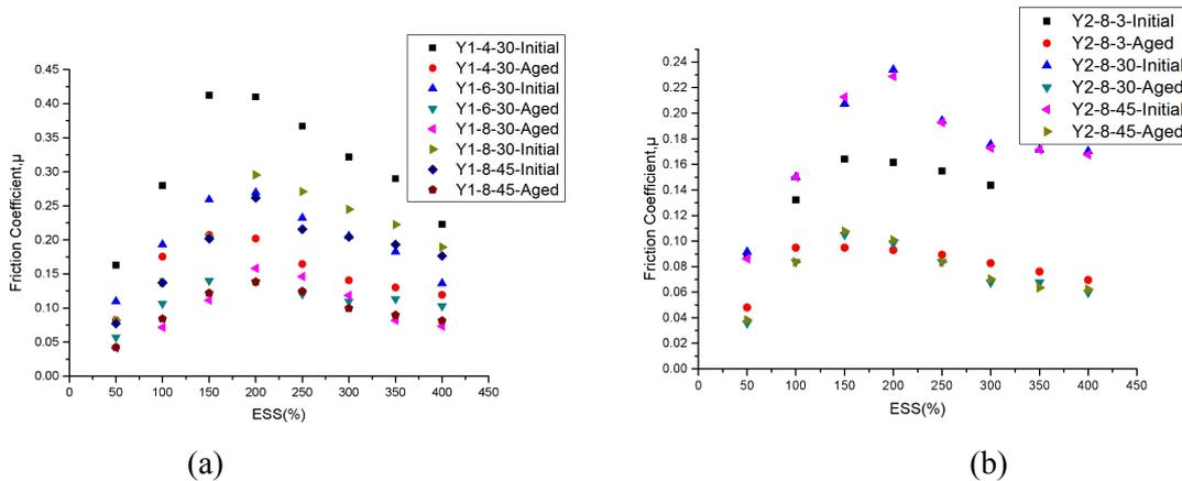
Fig. 6 - Observed friction versus increasing ESS: (a) Y1-Specimen; (b) Y2-Specimen.
