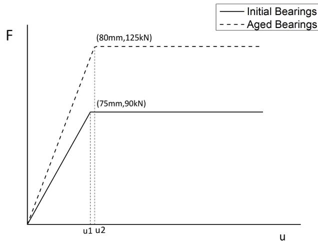
Fig. 7 - Mechanical model of SLEBs considering aged.
