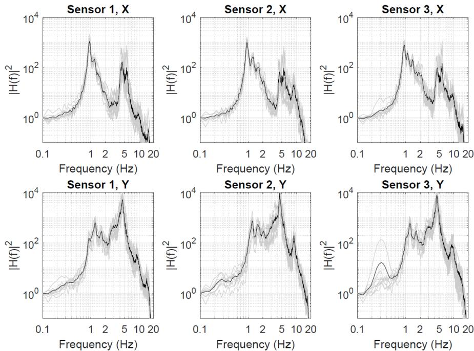
Fig. 2- Normalized amplitudes of complex frequency response function of the bridge estimated from Welch's average power spectral density function of traffic induced vibration. The gray lines correspond to 10 segments of the measurements and the black lines are their averages.
