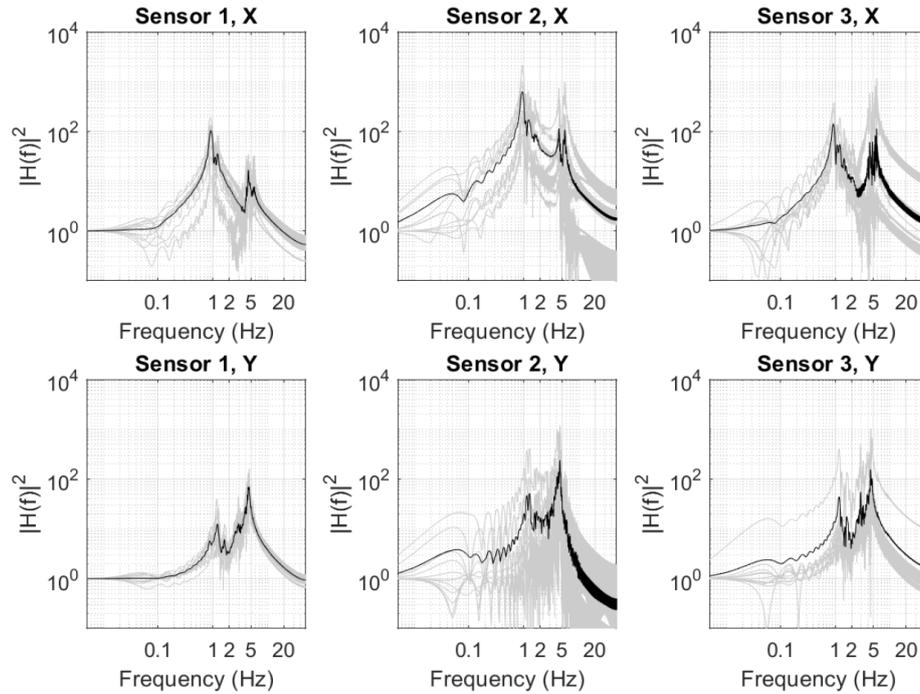
Fig. 3- Normalized amplitudes of complex frequency response function of the bridge estimated from the NEXt-ERA algorithm. The gray lines correspond to 10 segments of the measurements and the black lines are their averages
