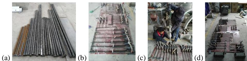
Fig. 3 - Manufacture process of test specimens: (a) the reinforcements cut off; (b) centered placed components; (c) grout pouring; (d) curing and hardening of grout
