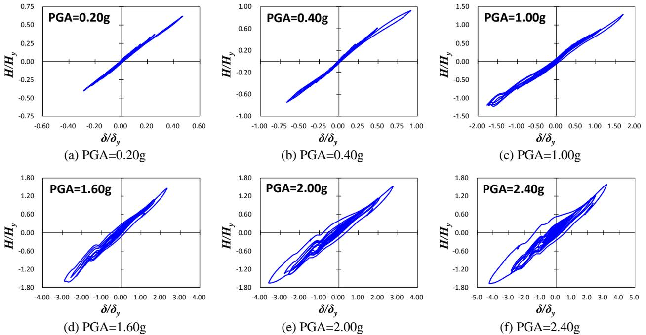
Fig. 6 – Hysteretic curves of the CFST-RC specimen under the seismic actions of Kobe Earthquake
