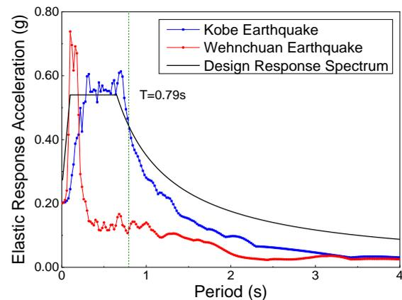
(b) Acceleration response spectrum of input ground motions with PGA=0.20g
