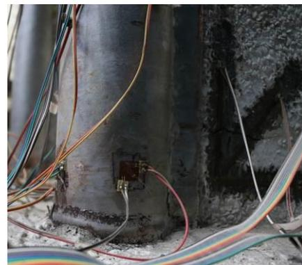
(b) Local buckling ring at the bottom of CFST limb
