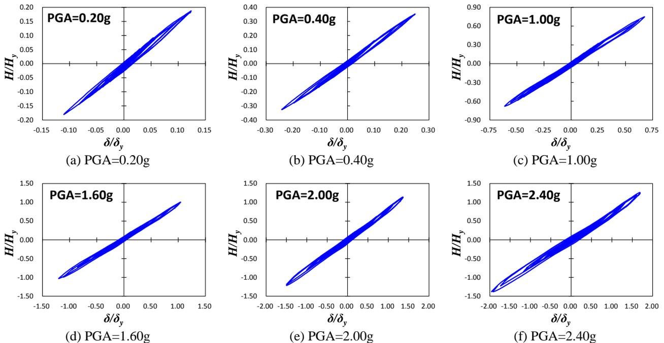
Fig. 7 – Hysteretic curves of the CFST-RC specimen under the seismic actions of Wenchuan Earthquake
