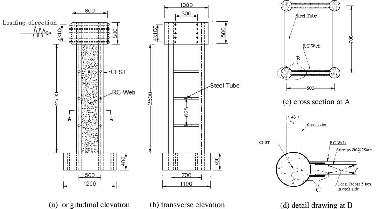
Fig. 2 – Details of CFST-RC column specimen (unit: mm)
