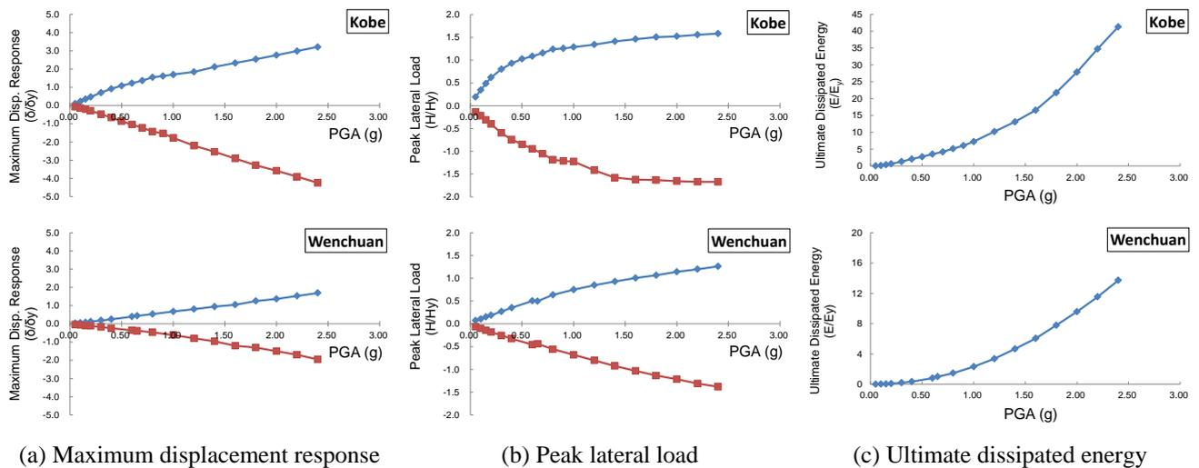
Fig. 10 – Change of seismic performance index with increase of ground motion intensity
