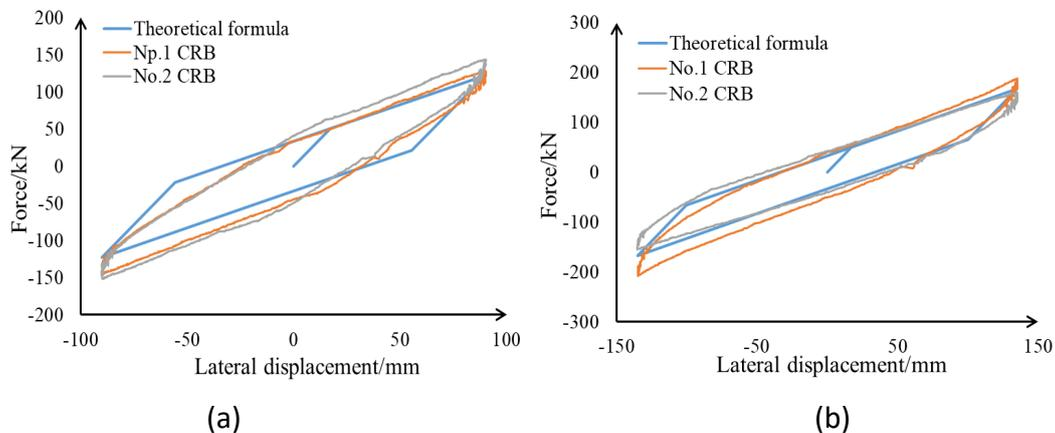
Fig. 5 – Theoretical hysteresis curves: (a) shear strain of 100%; (b) shear strain of 150%
