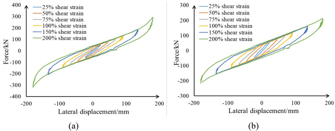
Fig. 4 – Quasi-static test results: (a) No.1 CRB; (b) No.2 CRB
