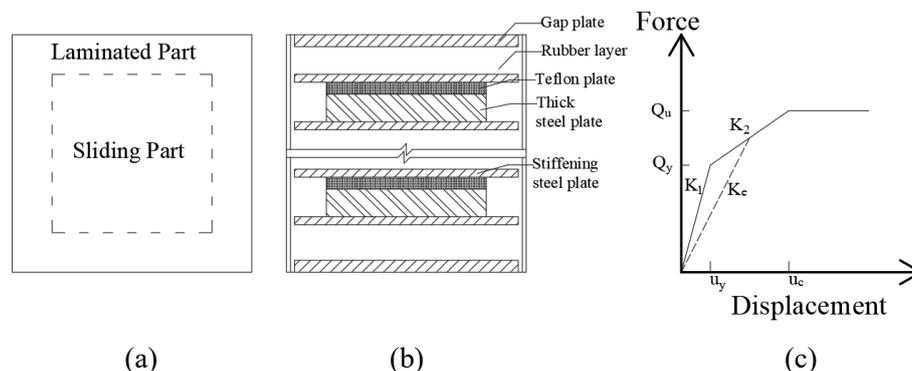
Fig. 1 – Composition of CRB: (a) plan; (b) elevation; (c) restoring-force model of CRB.
