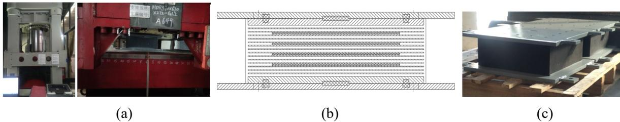
Fig. 2 – Experimental testing on CRBs: (a) testing machine; (b) profile of bearings; (c) full-scale specimens.
