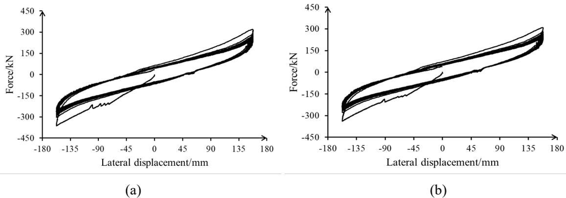
Fig. 3 – Horizontal equivalent stiffness test results: (a) No.1 CRB; (b) No.2 CRB
