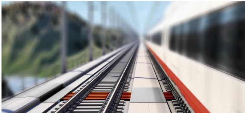
Fig. 15 – *Cross Tie* joint between single sections allowing longitudinal displacements with lateral, torsional and vertical off-set
