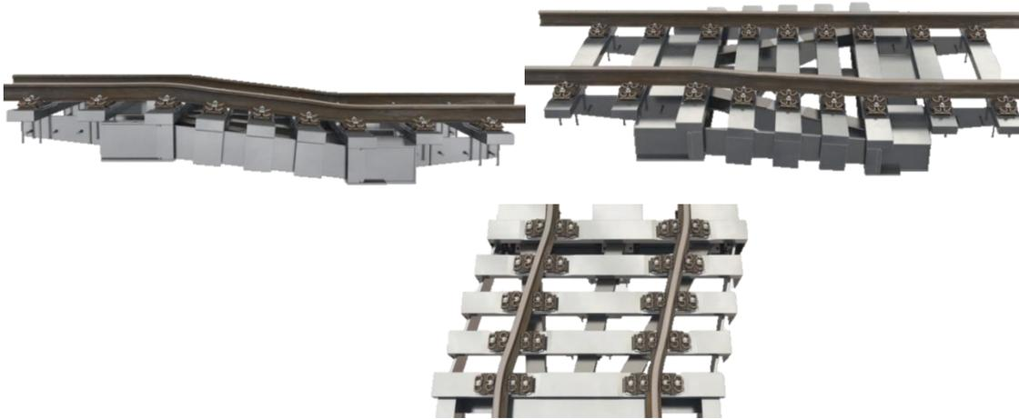
Fig. 16 – *Cross Tie* enables longitudinal displacements combined with lateral, torsional and vertical off-set
