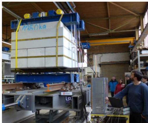
Fig. 17 – Dynamic full scale test of *Cross Tie* expansion joint
